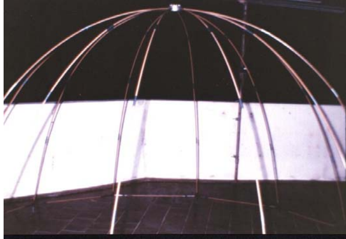
Figure 1: Camping tent, aluminum spline support structure.
