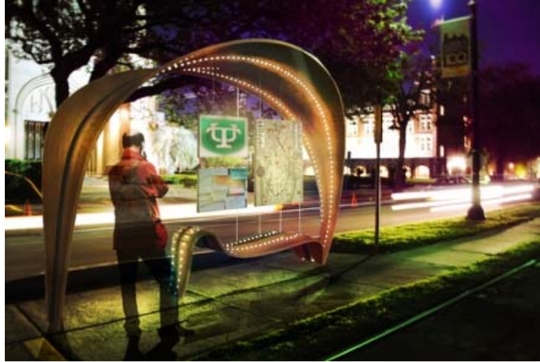
Figure 3: Tram station design. Wooden panels cover system. Steel pipe spline structure. https://www.behance.net/gallery/3542735/Cobra-Stop last accessed on 03.08.2015
