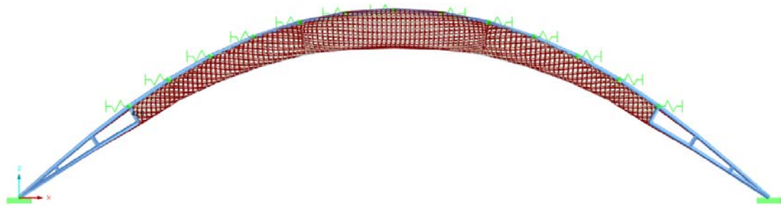
Figure 48: Spline arch plus pneumatic chambers (Final configuration) LOAD CASE 1 (DLUBAL RSTAB software)
