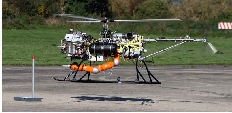
Figure 44: Autonomous helicopter with 7 DoF manipulator
