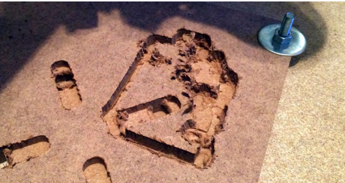
Figure 42: Slight vibration can rapidly increase and make the tool move around uncontrollably leading to potentially hazardous situations as cutters can break and be sent flying across the workshop. The consequences can be seen on this photo showing a failed milling of a part from medium density fibre board.
