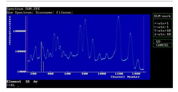
Figure 5.7: AXIL - KLM-Marker example of Ar ( $K\alpha$  and  $K\beta$ )
