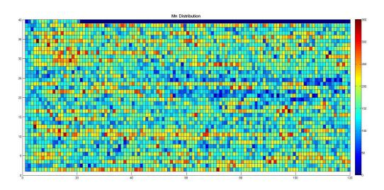
Figure 5.26: Detailed manganese (Mn) color map of the steel forging LP settings: 30s scan time, voltage of 40kV at  $80\mu$ A and a scan frame of 120x42 mm with a step size of 1mm. Mostly homogeneous distribution in contrast to the other elements Cr, Ni, Cu.
