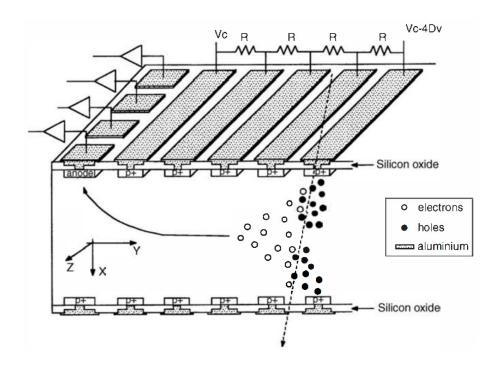
Figure 2.14: Cross section of a linear silicon drift detector (SDD)
