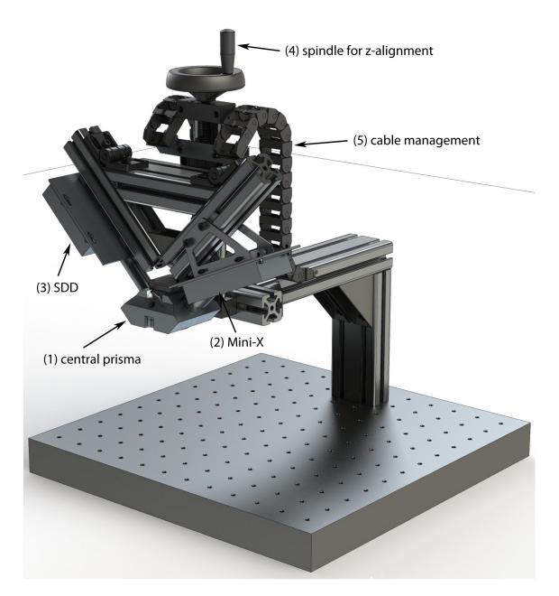
Figure 3.1: Final rendering of the Makro-XRF facility: (1) central prisma, (2) Mini-X X-ray source, (3) AXIS-D SDD, (4) spindle for z-alignment, (5) cable management
