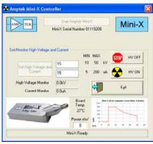
USB Software Interface. Allows the user to set the voltage and current as well as monitor both parameters.
