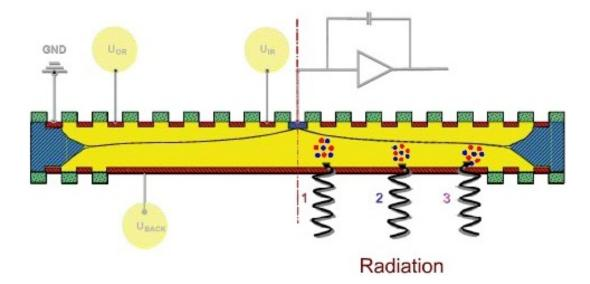
Figure 3.8: Working principle of a Silicon Drift Detector [1]:
