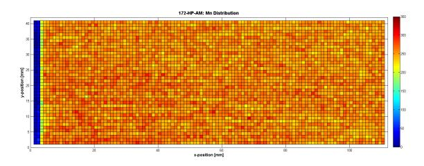
Figure 5.20: Detailed manganese color map of the 2nd section HPD settings: 5s scan time, voltage of 40kV at 5mA and a scan frame of 110x40 mm with a step size of 1mm. Mostly homogenous distribution.
