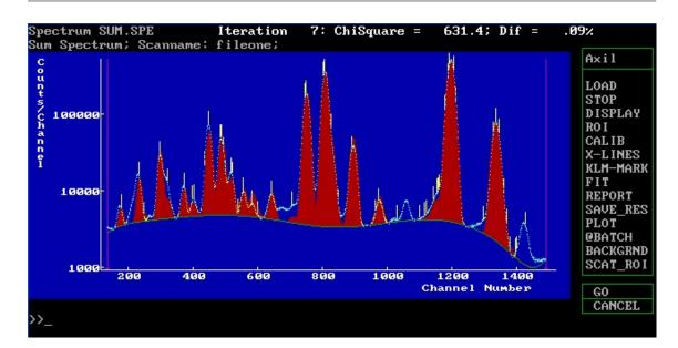
Figure 5.11: AXIL - Fitted spectrum, with information like the number of iterations, chi-square and the deviation between the last two iterations displayed on top
