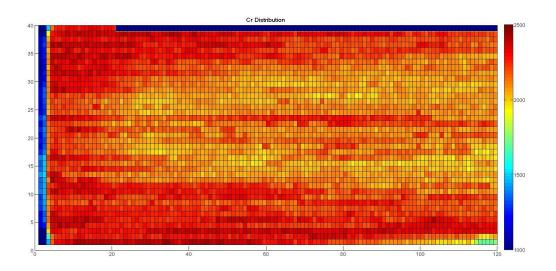
Figure 5.24: Detailed chromium (Cr) color map of the steel forging
