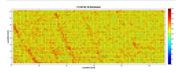
Figure 5.16: Detailed nickel color map of the 3rd section
