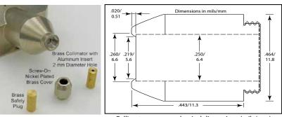
Collimator cover mechanical dimensions (mils/mm).
