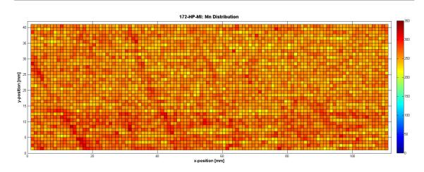
Figure 5.21: Detailed manganese color map of the 3rd section
