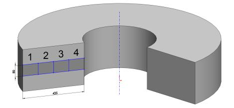
Figure 5.12: Ring forging from Breitenfeld Edelstahl AG [47]
