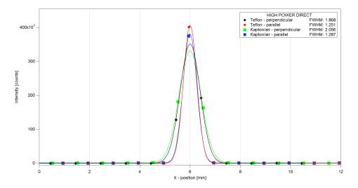
Figure 5.6: High power direct Gauss fits. Settings: 12mm line scan with a step size of 1mm, collimator Ø1mm, 20 seconds scan time and a voltage of 50kV at 35mA in either perpendicular or parallel orientation in respect to the copper wire, on a Kapton foil or a Teflon plate.
