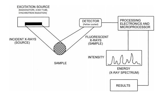
Figure 3.4: Schematic view of a basic XRF setup: A X-ray source irradiates the sample, resulting in characteristic X-ray radiation which is then measured by a detector and electronically processed to provide an energy/intensity spectrum for chemical analysis [21].
