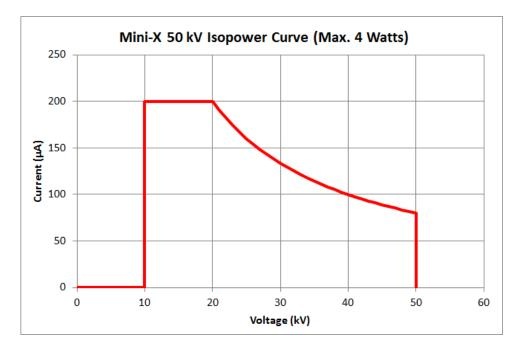
Figure 2.2: AMPTEK Mini-X isopower curve [3]
