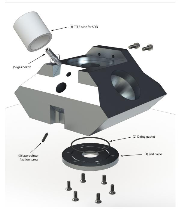
Figure 3.2: Central prisma: (1) end piece with optional Kapton [40] end window,(2) O-ring gasket, (3) laserpointer fixation screw, (4) PTFE tube for SDD, (5) gas nozzel
