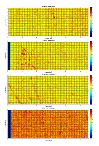
Figure 5.13: Elemental distribution of Ni from top=1 to bottom=4
