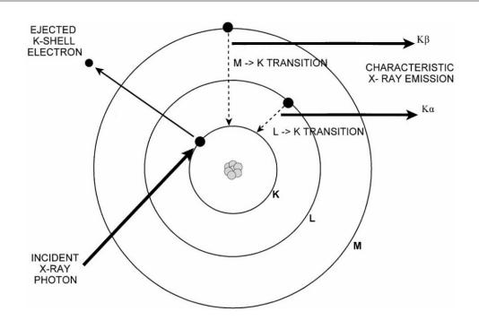
Figure 2.3: **Principle of XRF:** An X-ray of high enough energy excites an inner shell electron resulting in the emission of characteristic radiation as the vacancy is filled by an electron from an outer shell [21].
