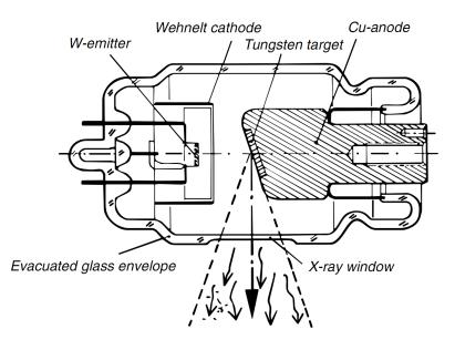
Figure 2.6: Basic principle of a side window configuration X-ray tube
