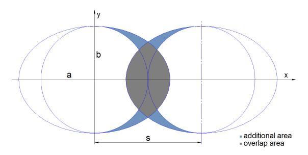
Figure 5.3: Different areas as a result of elliptic distortion
