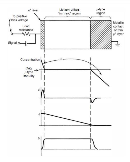
Figure 2.13: Basic principle of a lithium drifted p-i-n junction detector
