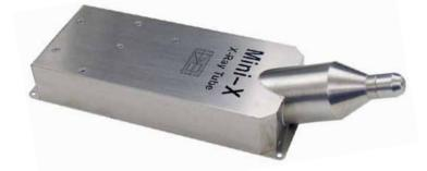
Mini-X is the first of its kind; a self-contained, packaged, miniature X-ray tube system, which includes the X-ray tube, the power supply, the control electronics and the USB communication to the computer. It is designed to replace radioisotopes in X-ray fluorescence analysis applications.
