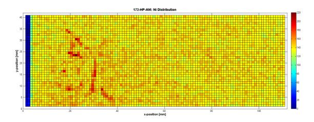
Figure 5.15: Detailed nickel color map of the 2nd section
