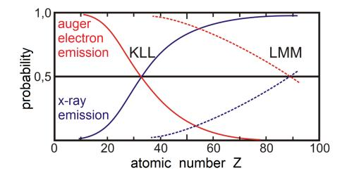
Figure 2.4: Auger versus X-ray emission probability
