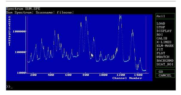
Figure 5.8: AXIL - example of several X-Lines added and represented as short yellow bars on top of the peaks
