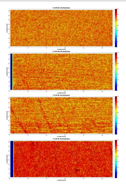
Figure 5.18: Elemental distribution of Mn from top=1 to bottom=4
