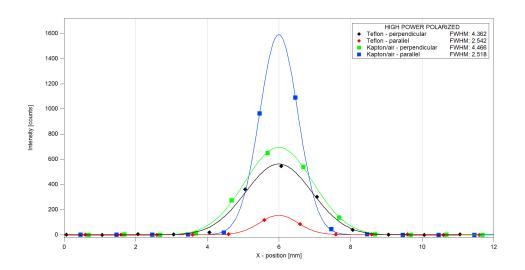
Figure 5.5: High power polarized Gauss fits. Settings: 12mm line scan with a step size of 1mm,collimator Ø1mm, 20 seconds scan time and a voltage of 50kV at 35mA in either perpendicular or parallel orientation in respect to the copper wire, on a Kapton foil or a Teflon plate.
