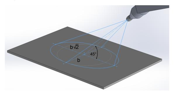
Figure 5.2: Illustration of the elliptic distortion of the beam spot
