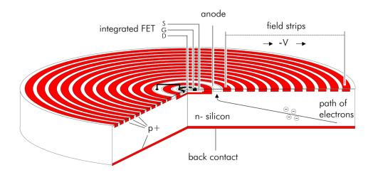
Figure 2.15: Cross section of a circular silicon drift detector (SDD)
