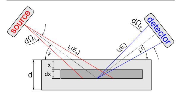
Figure 2.16: Geometry for the calculation of the intensity of characteristic radiation with the fundamental parameter method
