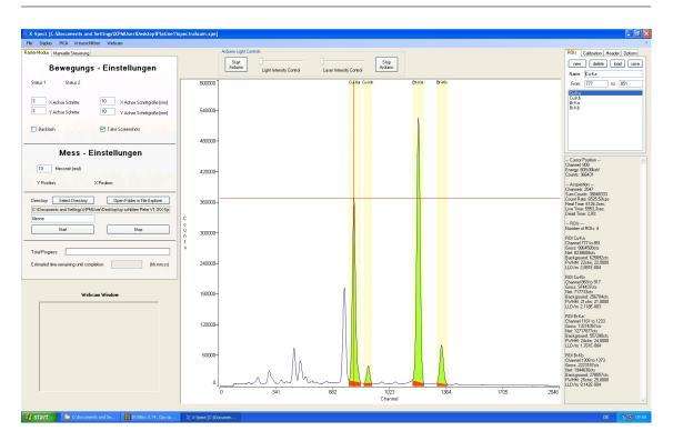
Figure 3.3: ROIs register depicting an example spectrum with several ROI's set and the corresponding information on the right
