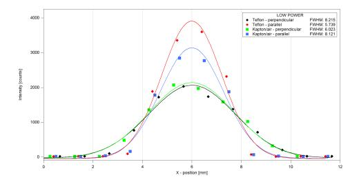
Figure 5.4: Low power Gauss fits. Settings: 12mm line scan with a step size of 1mm, collimator  $\emptyset$ 1mm, 20 seconds scan time and a voltage of 30kV at  $30\mu$ A in either perpendicular or parallel orientation in respect to the copper wire, on a Kapton foil or a Teflon plate.
