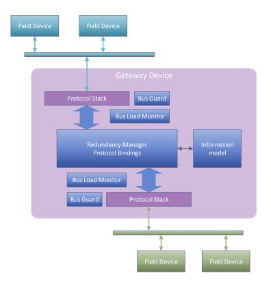
Figure 3.6: Gateway core components
