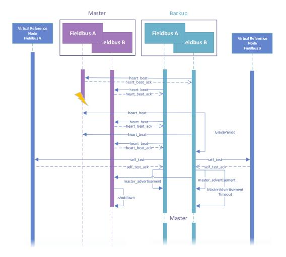
Figure 4.1: Link fault at *master gateway*
