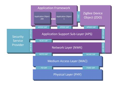
Figure 5.5: *ZigBee* architecture [29]
