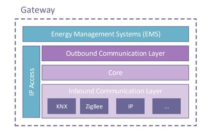
Figure 2.8: EEBus gateway architecture
