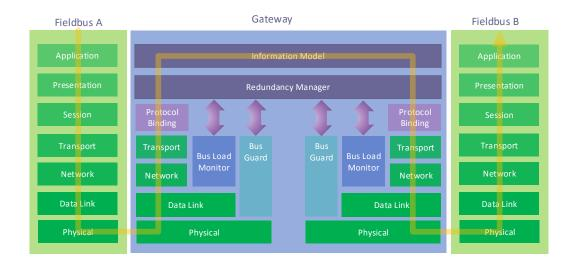
Figure 3.5: ISO/OSI 7 layer model incorporating a gateway
