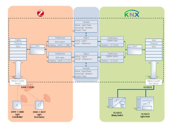
Figure 5.11: Information model of evaluation testbed
