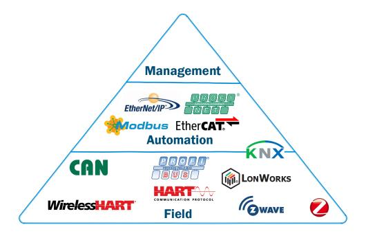
**Figure 1.1:** Automation pyramid for BACS according to *ISO 16484-2:2004* [11] illustrating the heterogeneity of the field layer
