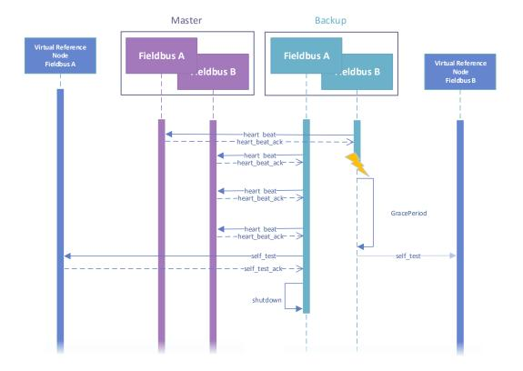
Figure 4.3: Link fault at *backup gateway*
