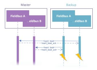
Figure 4.4: Device fault at backup gateway
