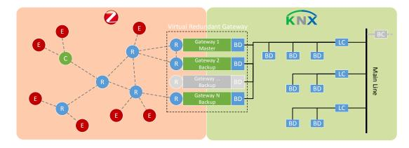
Figure 5.1: KNX-ZigBee gateway schematic overview
