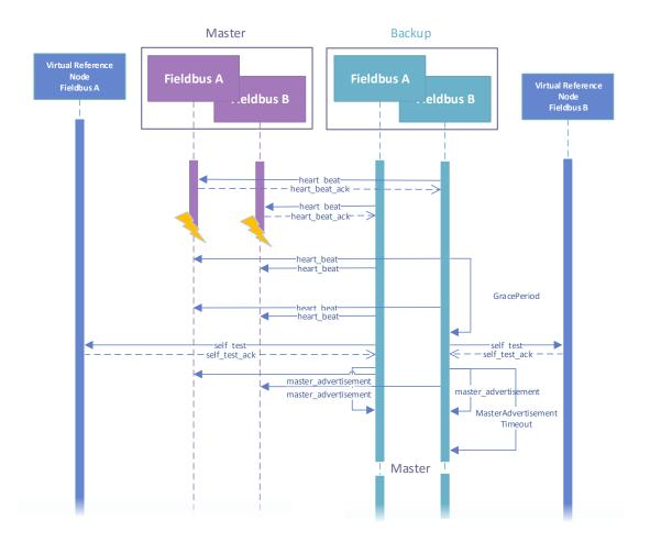
Figure 4.2: Device fault at master gateway
