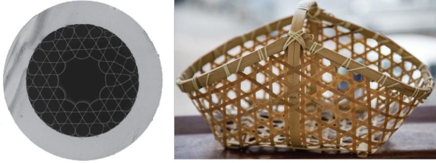
Figure 7.1: A SEM image of Kagome lattice HC-PCF. The name “Kagome” is composed from the words *kago*, meaning "basket", and *me*, meaning "eye" and it comes from a traditional Japanese woven bamboo pattern that is used to make baskets.
