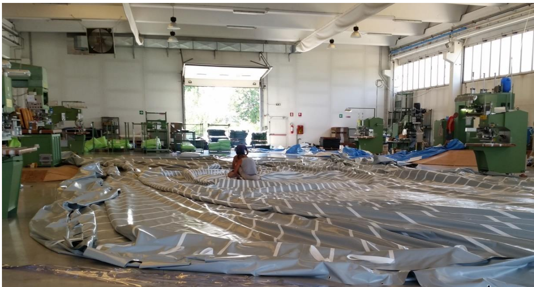
Picture 1. View of a conical PVC membrane cover under welding at the author production shop with workers finishing the hot air welding of PVC coated belts over the main cover membrane
