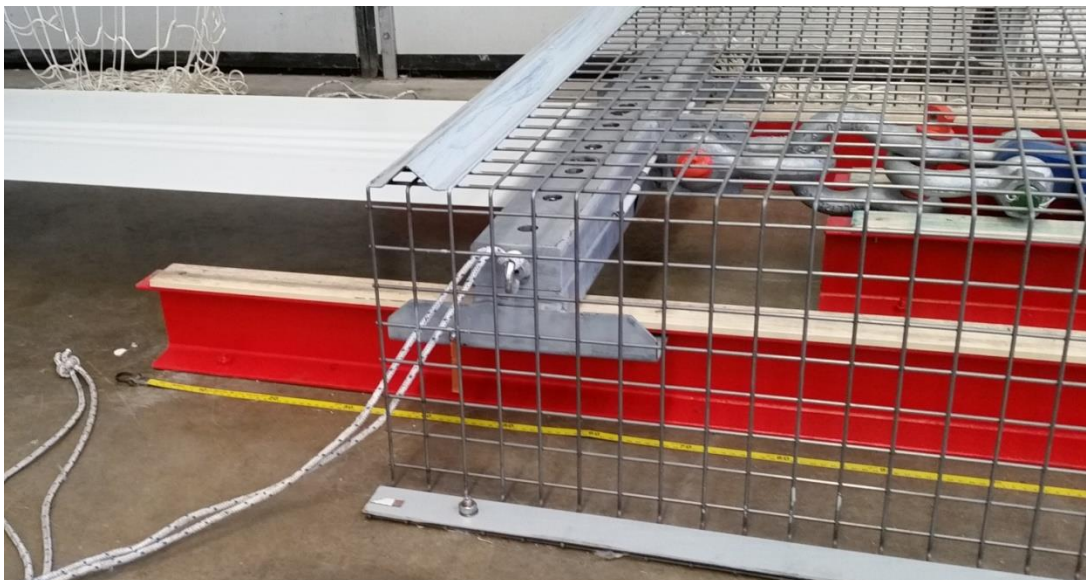
Picture 6. View of part of the testing machine moving anchor flange that slides over the red colored rails coated with a smooth wooden top. The metric long metal ruler that serves to measure the sample elongation under the tensile force can also be seen.
