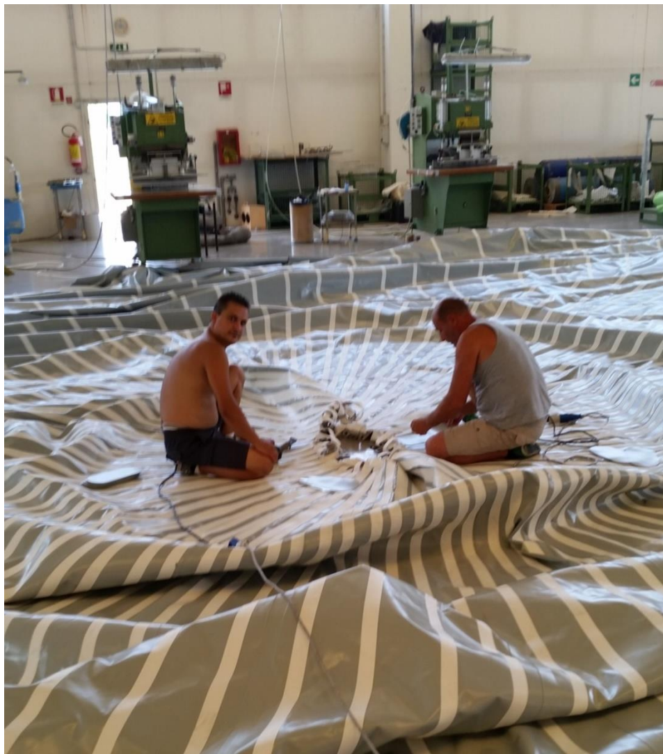
Picture 2 View of the conical shaped cover centre with all the belts ending in a stainless steel buckle to be bolted to a steel central anchoring flange placed on the top of a steel central mast. It can be seen the high complex work of the technician that has to carefully connect all the edges of the belts in the right position in order to correctly execute the bolting in the right places.
