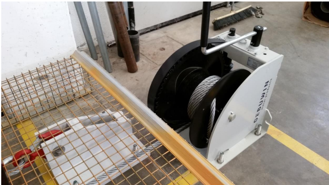
Picture 7. View of the manual winch able to execute a max traction force of 5 T
