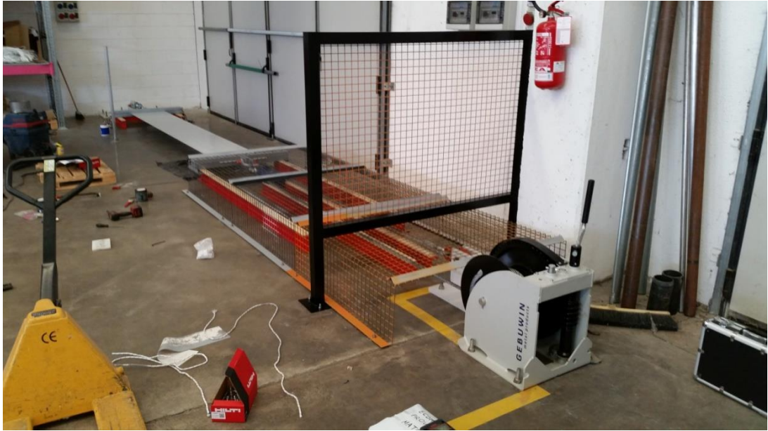
Picture 8. View of the full testing machine on the side of the winch. All the safety steel mesh protection screens can be clearly visible.
