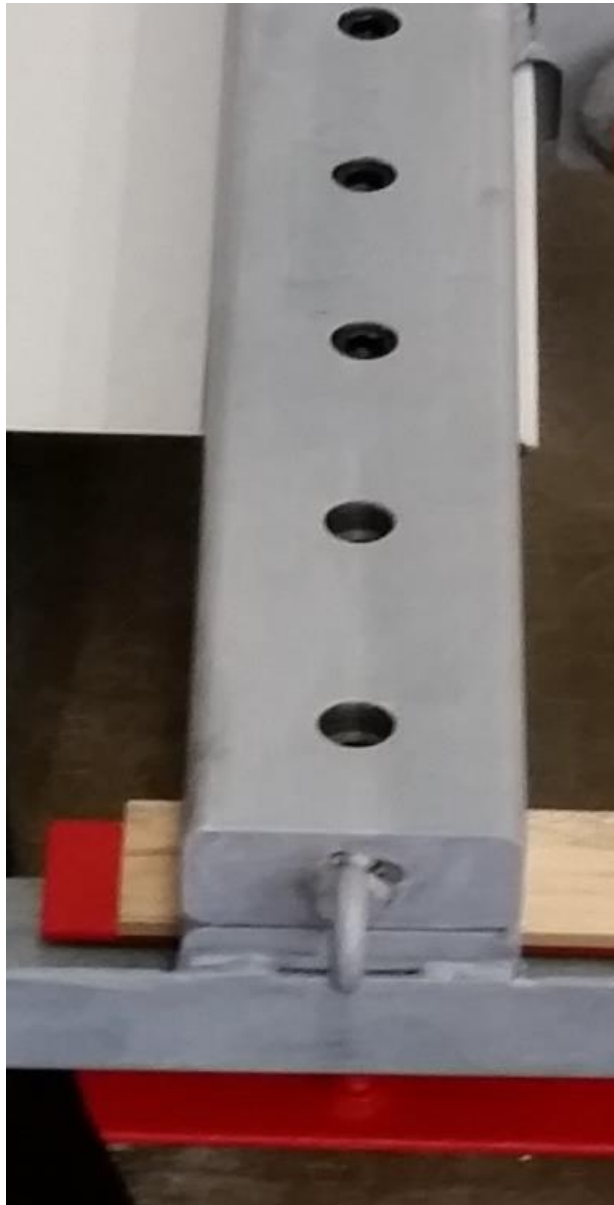
Picture 5. View of the smoothed section of the anchoring flanges and of the safety steel flaps placed underneath the moving flange to let the bolted profile slide over the steel railings without the risk of moving randomly at the time of the sample test breaking point.
