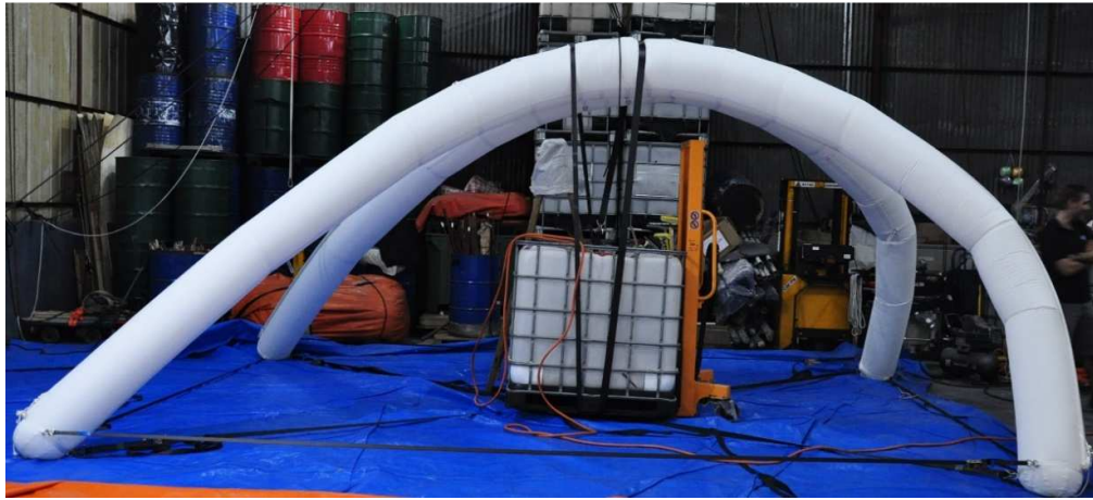
Figure 74. Test configuration under point load demonstrating longitudinal buckling mode. (By author)
