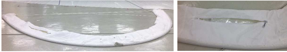
Figure 69. Inner TPU bladder inserted into the outer sleeve with the GFRP rods inserted and bent. (By author)
