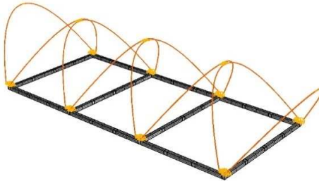
Figure 60. Bending-active element fixing strategy. (By author)
