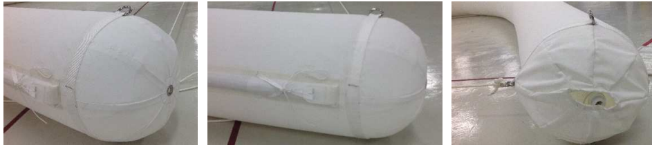
Figure 71. Termination of the tube with GFRP and valve on one end. (By author)
