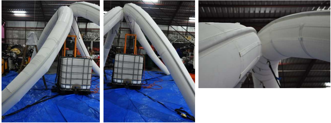
Figure 78. Twist buckling mode observed and rotation at apex. (By author)
