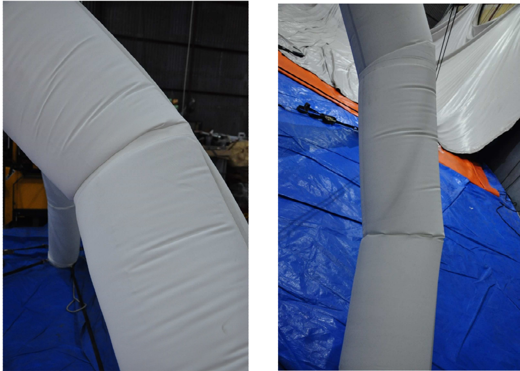
Figure 76. Test configuration, compression folds under point load. (By author)
