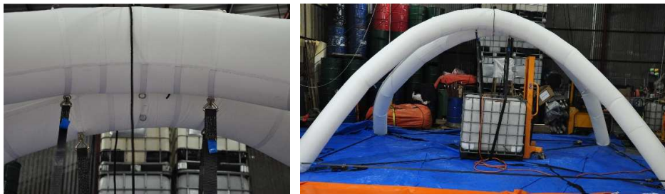
Figure 77. Point load changed to below tube and resulting twist buckling mode. (By author)
