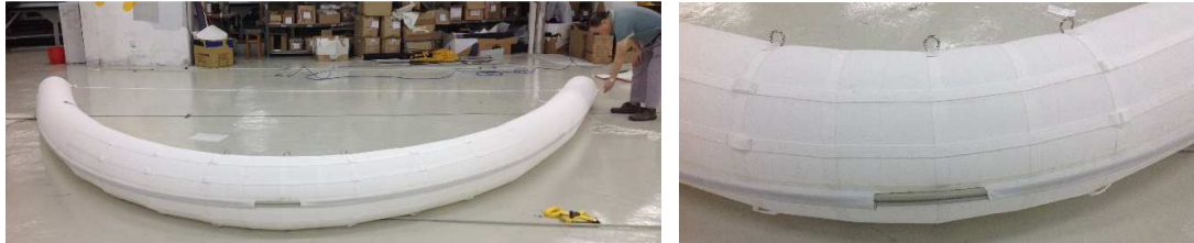
Figure 70. Inner bladder inflated with two GFRP rods with bottom tension cord in place. (By author)
