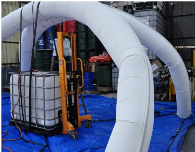
Figure 75. Test configuration under point load, GFRP component in bending deformation. (By author)
