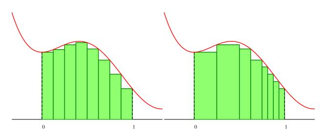
FIGURE 1. Numerical integration of some given function with uniform grid (left) and adaptively generated (grid).
