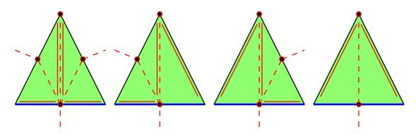
FIGURE 1. Refinement rules for 2D bisection (newest vertex bisection). The reference edge is indicated in blue. The leftmost triangle depicts the *bisec3* refinement of a marked element. The other three refinement rules (*bisec2* and *bisec1*) are recursively applied to avoid hanging nodes. The dashed line outside of the triangles indicates where the neighboring triangle is refined.
