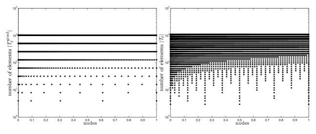
FIGURE 3. Graded partitions with  $\beta = 4/3$  (left) and adaptively generated partitions (right). Each row shows the nodes of a partition  $\mathcal{T}_{\ell}^{\text{grad}}$  resp.  $\mathcal{T}_{\ell}$  in the interval [0, 1]. The height of the row indicates the number of elements in the particular partition.
