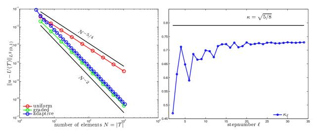
FIGURE 2. The left-hand side figure compares uniform refinement, graded partitions, and adaptively generated partitions to approximate  $u(x) := x^{-1/4}$ . The right-hand side figure shows the experimental contraction constant  $\kappa_{\ell} := \operatorname{err}(\mathcal{T}_{\ell})/\operatorname{err}(\mathcal{T}_{\ell-1})$  as well as the theoretical bound  $\kappa = \sqrt{5/8}$  for adaptive refinement.
