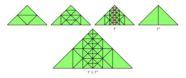
FIGURE 3. Counter-example to (2.5.1) for red-green-blue refinement. With j = 4, there holds  $|\mathcal{T} \oplus \mathcal{T}' \setminus \mathcal{T}| = 4j$  and  $|\mathcal{T}'| = 2$ . Obviously, the construction can be extended to any  $j = 2^n$ ,  $n \in \mathbb{N}$  by red-refinement of the marked triangles in  $\mathcal{T}$  and thus contradicts (2.5.1) for any constant.
