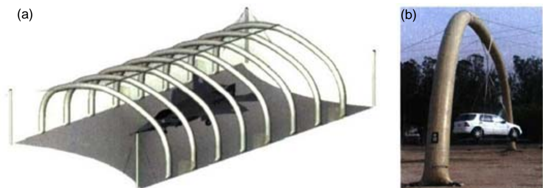
Figure 3 - 27: (a) Inflated fabric arches used in aircraft shelters; (b) Demonstration of an arch load carrying capability. 31
