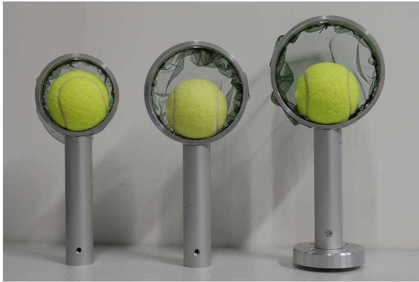
Figure 4.23: Catching devices with the same distance of the center of the ring to the mounting flange and different ring diameters (80 mm, 100 mm and 110 mm)
