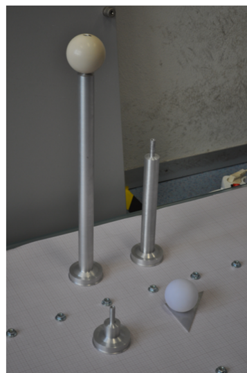
(b) Stands for the sphere used for the camera accuracy experiments; three stands with different heights (80 mm , 280 mm and 480 mm ) for experiment with the external illumination, stand with triangle-shaped base with self illuminating sphere.
