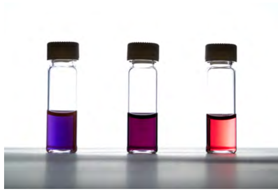
Figure 3.9: Monodispersed gold nanoparticles. Photograph of monodispersed gold nanoparticles in deionized water. The color of the colloid depends on the size of the nanoparticles. By decreasing the nanoparticle size from left to right, the color changes from blue to red. The photograph was made by A. Bellew [95].
