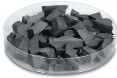
Figure 4.16: Indium tin oxide (ITO) pieces for physical vapor deposition. Indium tin oxide (ITO) pieces as they are used in physical vapor deposition or electron beam deposition. In bulk form, they are entirely opaque. (The image is taken from www.lesker.com .)
