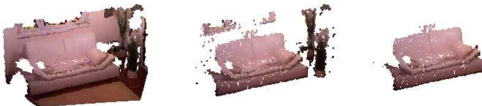
Figure 3.27: From left to right: Extracted point cloud resulting from the 2D object detection, 3D cluster extraction and the final point cloud after Euclidean clustering.
