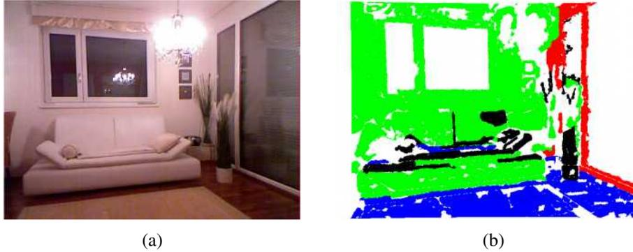
Figure 3.7: Initial labeling. (a) RGB input image. (b) Detected ground plane and wall segments obtained by the labeling algorithm.
