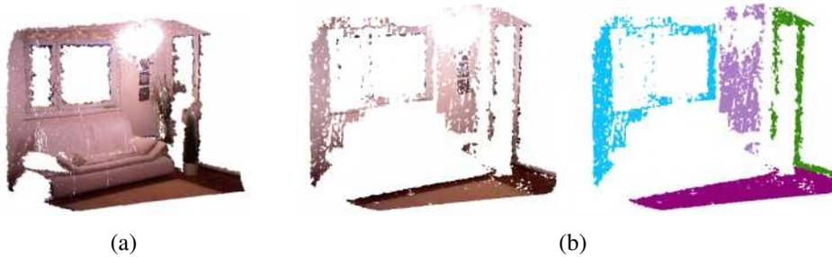
Figure 3.8: (a) Raw 3D point cloud. (b) Walls detected by the super-pixel labeling / plane-fitting algorithm.
