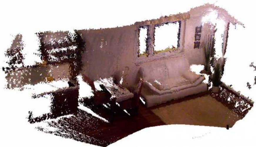
Figure 3.6: Multiple point clouds are stitched together to generate a dense point cloud of the RGBD video.
