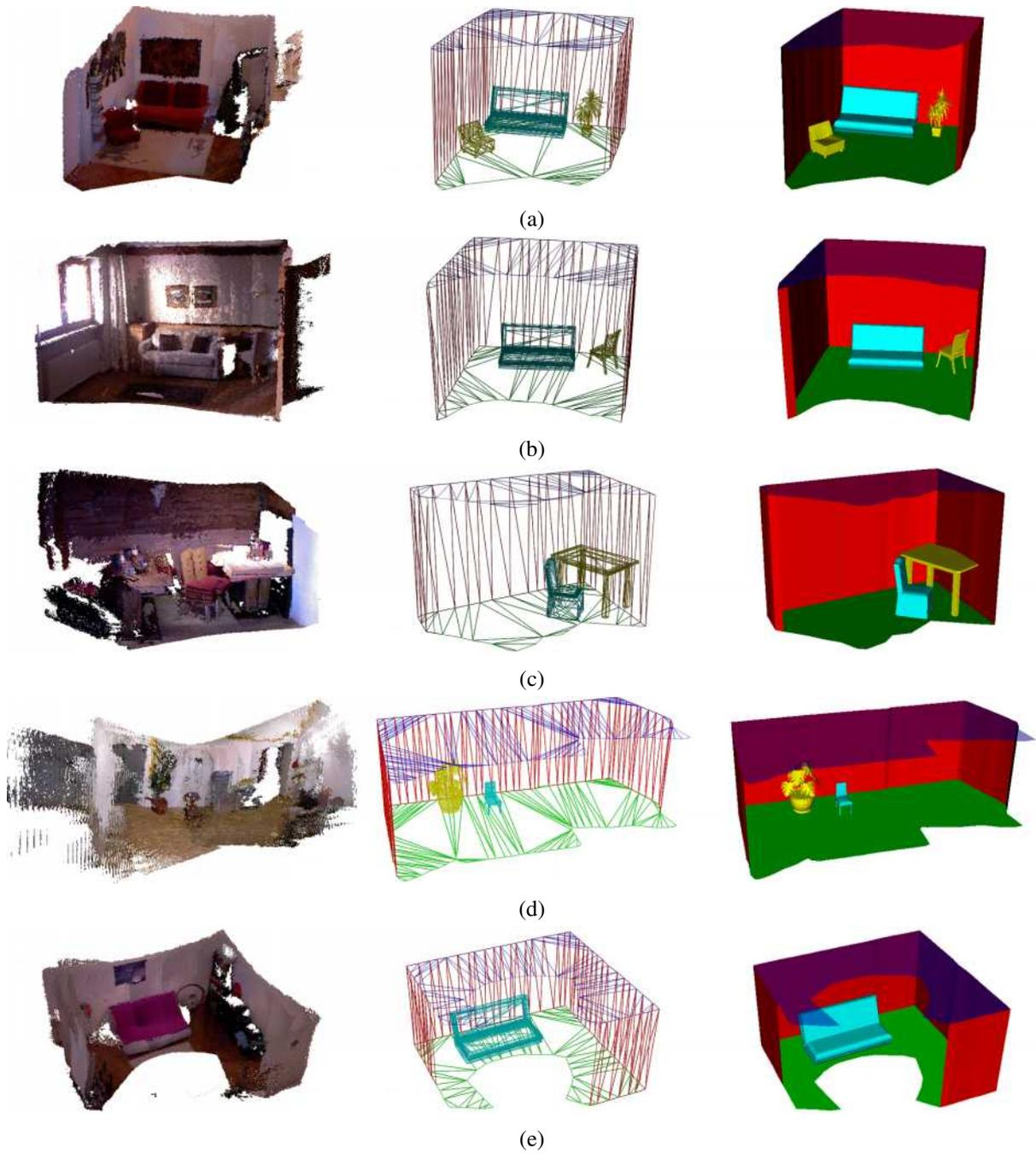
Figure 4.13: Optimized results for the sample videos (1-5). A RGBD video sequence is used to create a dense point cloud (column 1). The proposed framework estimates a mesh-based, smooth and simplified model of the scene with a limited number of vertices and faces (column 2 and 3). Each sample shows the MRF optimized object classification result.
