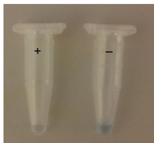
Fig. 24 Evaluation of the coupling efficiency with an immunoassay approach. (+) indicates the reaction of AFB 1 modified beads – a color change was expected due to the use of an anti-aflatoxin antibody. (-) shows the reaction of unmodified beads; no color change was expected.
