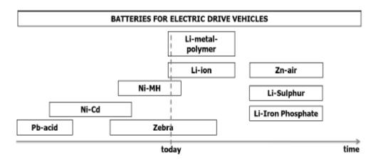
Figure 8: Batteries for electric vehicles (Source: Norwegian University of Science and Technology, Nina Wahl Gunderson, 2010)
