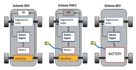
**Figure 4: Electric vehicle types** (*Source: CSCanada*<sup>25</sup>)
