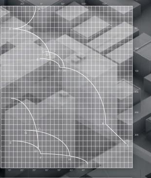
Predefining the optimal siting for the nucleus inside the host building. The field diagram shows the best direction for the nucleus to develop. Structural and statical analysis of the building serve as foundation for this analysis. Weaker areas of the building means better areas to develop but they are also carry less load.
