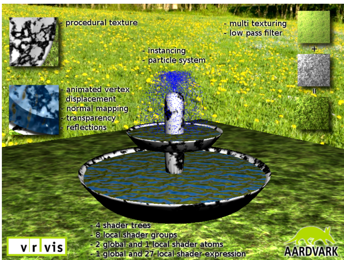
Figure 5.1: The fountain example includes four shader trees for procedural marble, animated water, low pass filtered grass, and an instancing particle system for water droplets.
