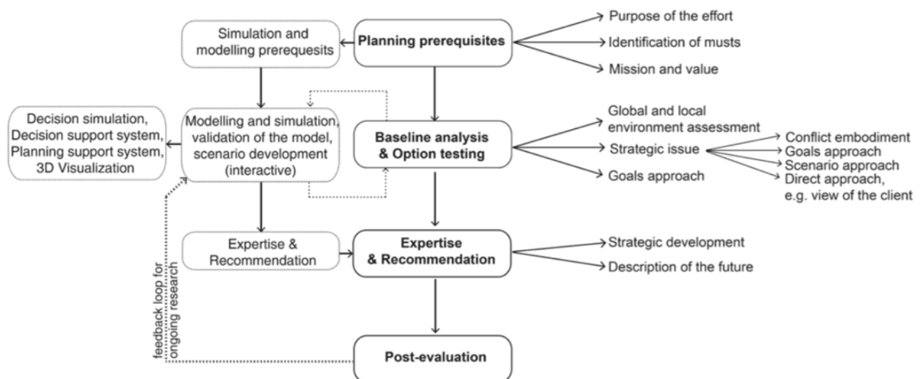
Figure 1. A strategic planning process incorporating a simulation and modelling process, in the Routledge Handbook of Planning Research Methods p. 351(Yamu, 2015)
