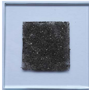
Fig. 20: Finished XRD sample on a glass carrier of 5 x 5 cm and the powder was placed on a 3 x 3 cm area in the middle of the glass carrier.
