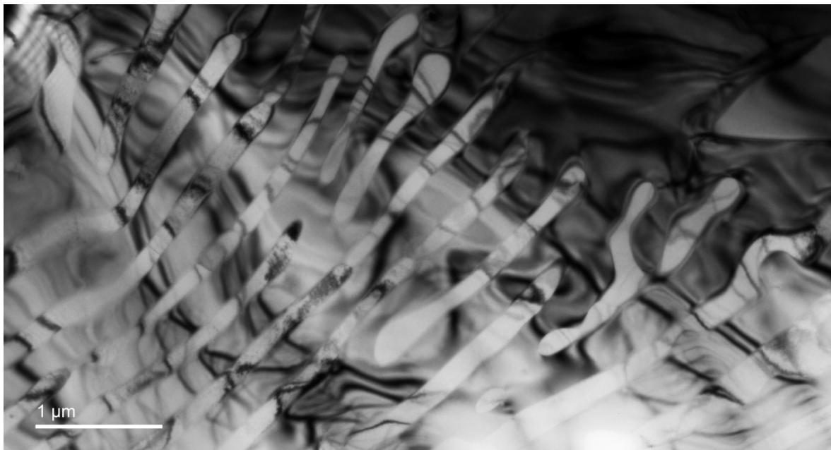
Fig. 40: Bright field image of the cast material including precipitates with different phase.
