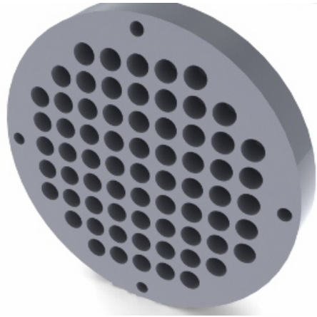
Figure 2.5: The figure shows an example for a hollow cathode design [16].
