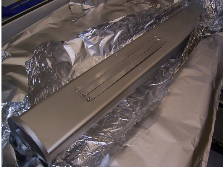
Figure 3.8: Image of the three sample stripes mounted on a liner facing the stripe detector.
