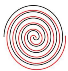
Fig. 2-59: Mechanism of a scroll pump
