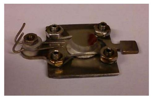
Fig. 7-21: Sample holder with bended alumel/chromel thermocouple wires.
