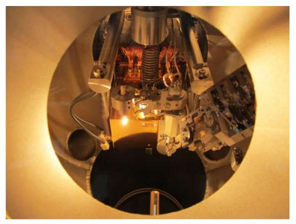
Fig. 7-17: Picture of the STM unit mounted in the vacuum chamber. The filament tower (glowing filament) can be used for sample heating during measurement. Small saphire balls are used for thermal insulation between sample holder and STM electronics.
