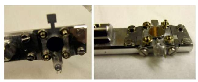
Fig. 3-65: Sample plate and transfer holder of the HP-XPS system. The transfer holder is used to move the sample from the load lock to the UHV chamber. Due to the arrangement of the vacuum chamber, transfer steps cannot be observed through a viewport, but could be observed by a camera.
