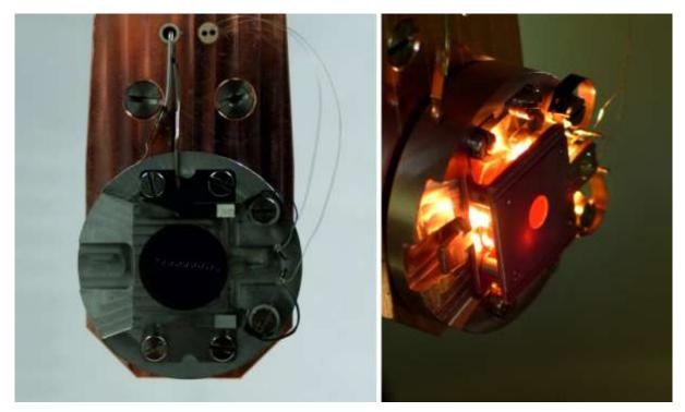
Fig. 2-51: E-beam heater of the STM system. Left: filament; right: glowing filament with sample.
