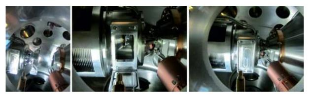
Fig. 2-28: HP-XPS cell. On the left side with open bayonet coupling to the analyzer, in the middle open sample inlet and on the right side ready for measurement.
