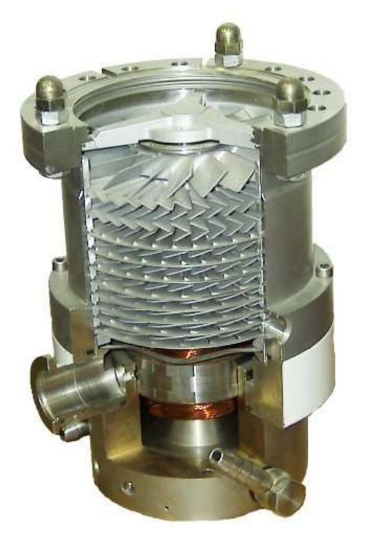
Fig. 2-61: 3D model of a turbomolecular pump [131].
