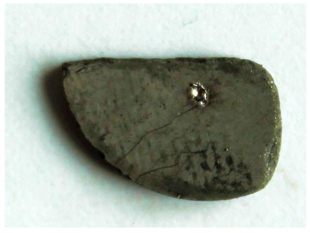
Fig. 4-27: Picture of the  $Pd_2Zn$  pellet. The surface is rough and non-uniform, also some contaminations/enclaves in the bulk can be seen.
