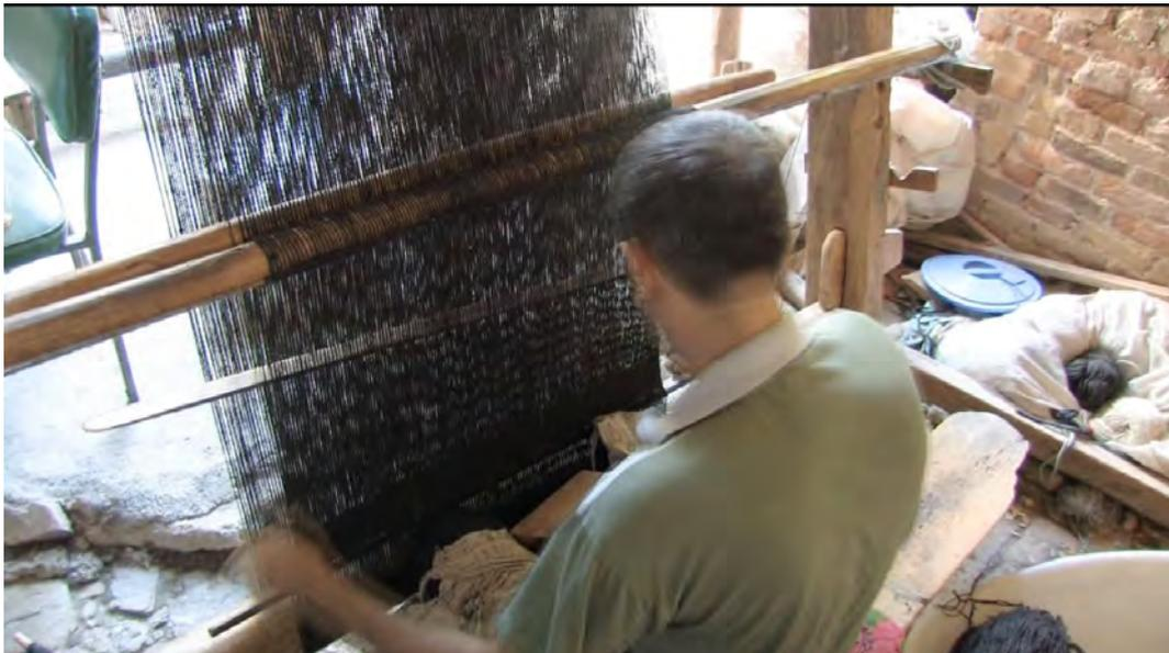
*image 4.090: After the threading of the rod heddle is completed, the shed rod is stuck into the warp behind. Below, the sword beater can be seen. The weaver is about to drive a bobbin through the warp starting the weft. At the back of the lower beam the metal warping rod being fixed at the end of the weft can be seen. Now, during the weaving process, it will slowly move upwards with the weft at the back of the loom.*
