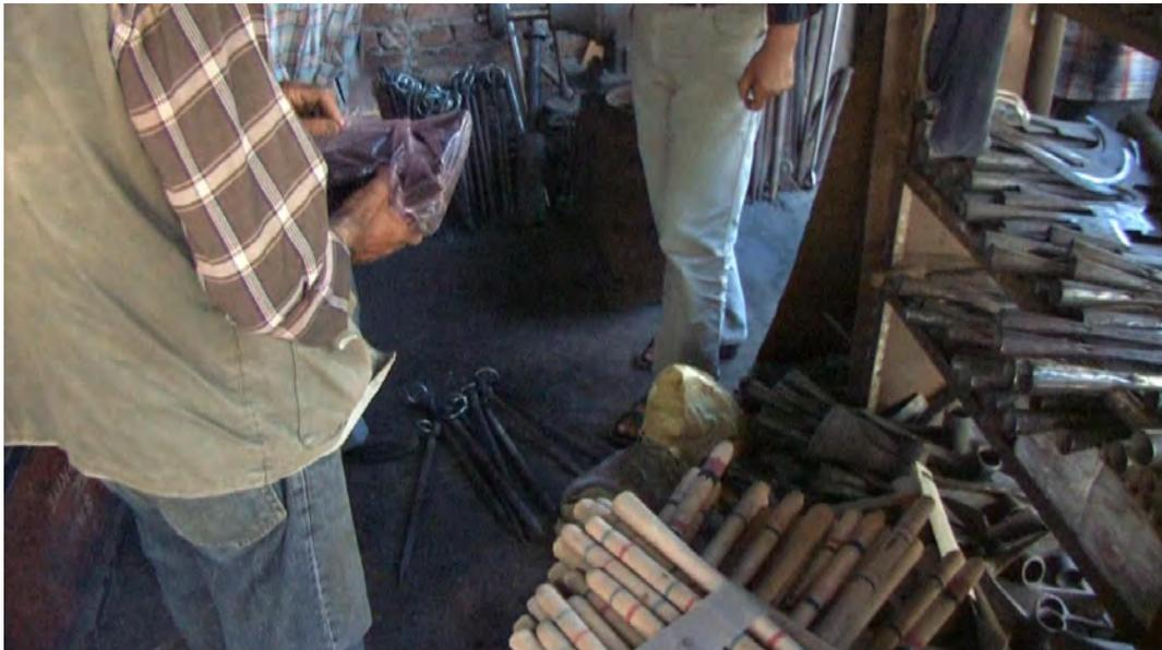
*image 4.012: In the middle, on the floor, the eight stakes can be seen which were made from structural steel bars.*
