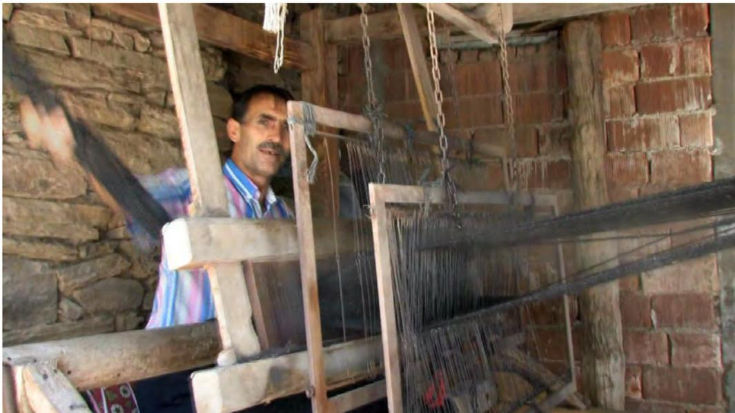
*image 4.093: The heddle harnesses open and counter-open the shed.*
