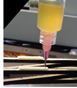
Figure 3.77: Applying glue on the protruding edges
