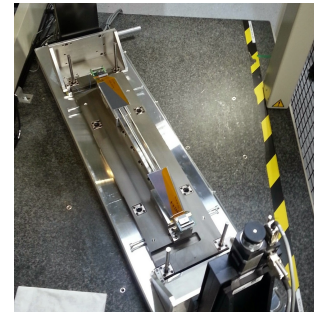
Figure 3.53: backward and forward sensors glued to rib
