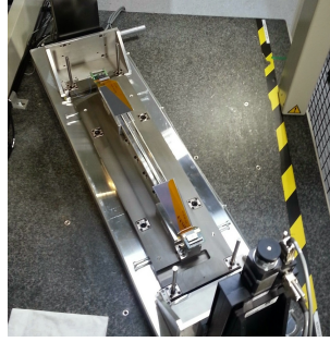
Figure 3.76: Rib assembly on assembly base on CMM surface
