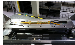
Figure 3.80: Assembly bench lowered to rib assembly
