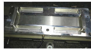
Figure 3.63: Gluing thermal insulator to sensors
