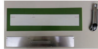
Figure 3.60: Cut out Thermal insulator sheet 'Airex'
