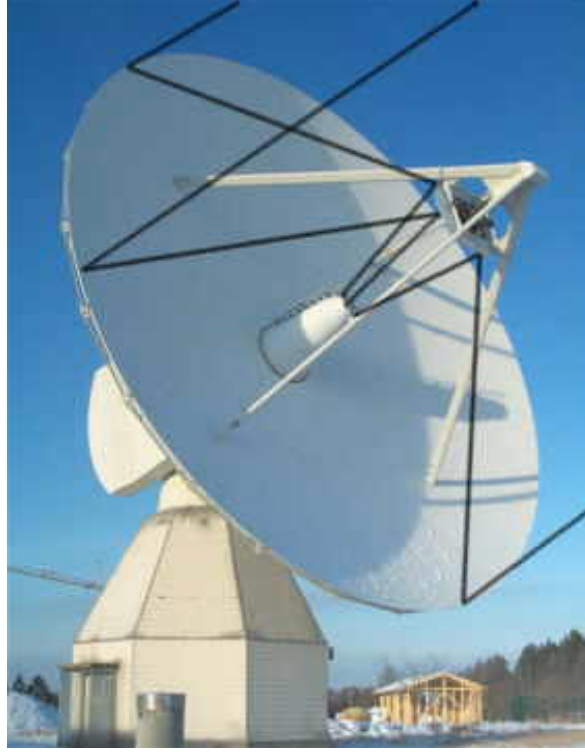
Figure 2.3: VLBI 20 m antenna from the fundamental station Wettzell a with signal path.
