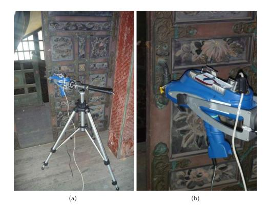
Figure 10.3: Setup for the measurement of the brass handle in the first floor. (a) overview, (b) detail.
