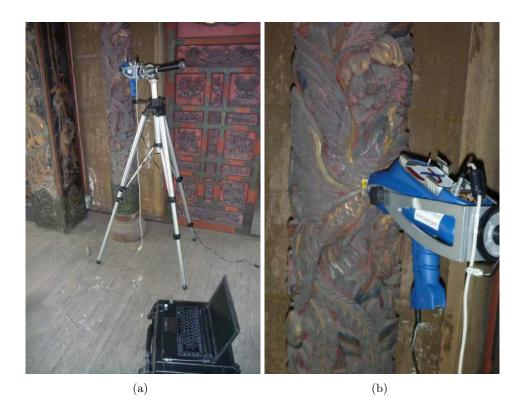
**Figure 10.2:** Setup for the measurement of the wooden column in the fourth floor. The dark red color probably stems from  $Fe_2O_3$  in Armenian clay, that is used during gilding. The gold layer can also be seen in the better preserved cavities and narrow gaps. (a) overview, (b) detail.
