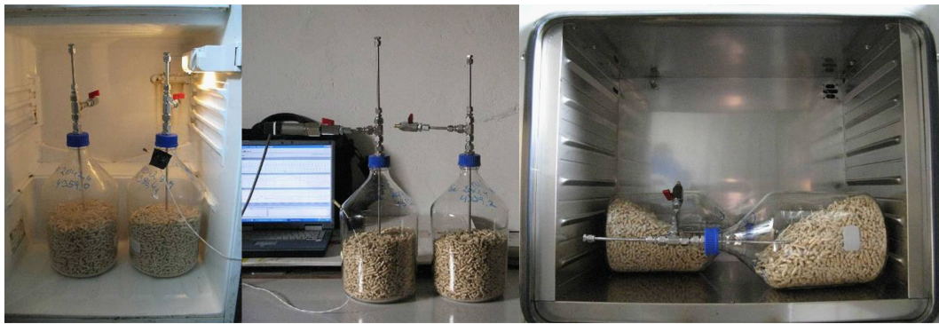
Figure II.9.: Experimental setup for the investigation on the influence of storage temperature and storage atmosphere, from left to right depicting the storage at 7, 20 and 50 °C.
