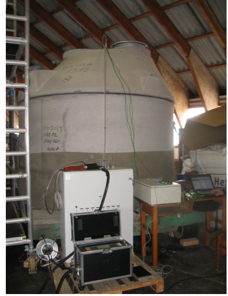
Figure IV.4.: Experimental setup of the concrete tank in the storage depot. In front of the tank the gas analyzer and the switch board for the measurement cycle can be seen.
