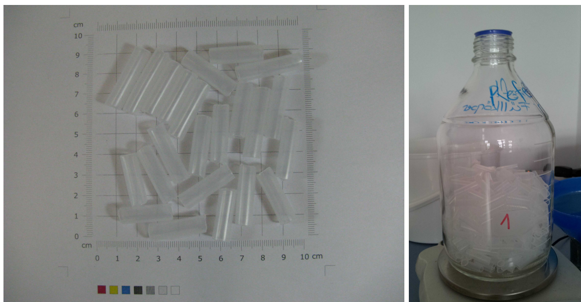
Figure II.18.: On the left a picture of the LD-PE filling material and to the right the 2-liter glass flasks with the filling material.
