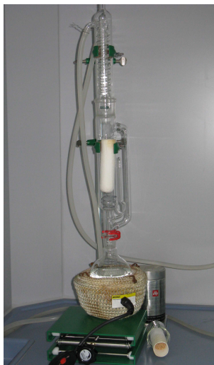
Figure II.2.: Soxhlet extractor with extraction thimble placed inside.
