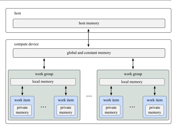
Figure 2.3: The OpenCL memory model illustrates the different memory regions within the host and the compute devices [Gro].
