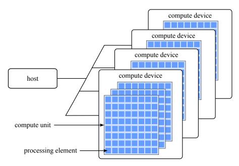
Figure 2.1: The OpenCL platform model consists of a host application that controls various compute devices. A compute device consists of numerous compute units that are divided into processing elements [Gro].
