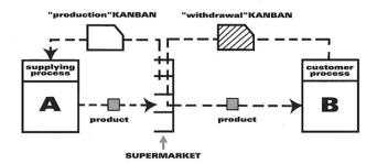
Figure 3.9 Example of a Pull System by using Supermarket with Kanban (Today's Lena manufacturing 2011, www.todaysleanmanufacturing.com)
