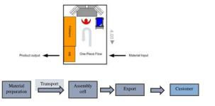
Prepare material and assembly in One Piece Flow 3 products according to working instructions. Another participant measures the time of material preparation, production, functional testing. The trainer writes the time into the table.
