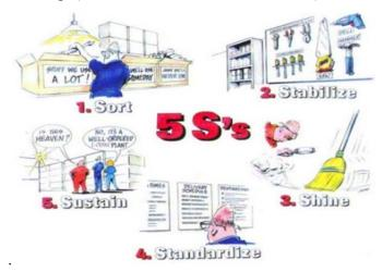
Figure 3.2 Five steps in 5S Method (E-Crane Worldwide 2014: www.e-crane.com)
