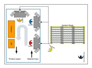
Figure 8.13 U-Cell with 3 Workstation and Kanban system
