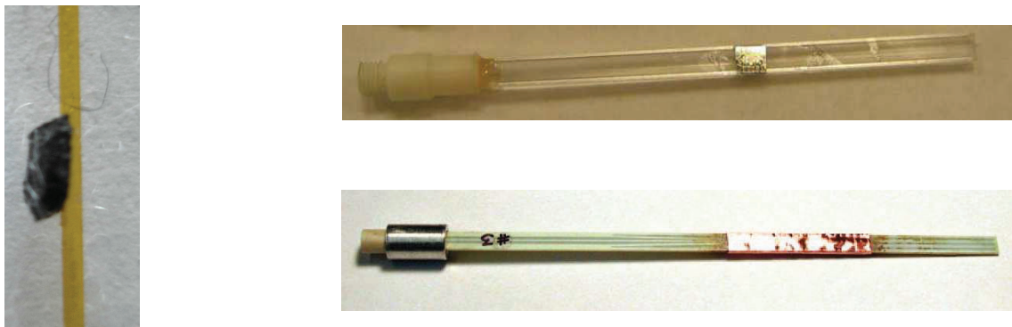
Figure 3.2: The left panel shows a photograph of a mounted \text{CeRu}_4\text{Sn}_6 sample on the sample holder for SQUID measurements. The right panel displays the two sample holders used in the PPMS. On top the low temperature quartz sample holder with a mounted sample is shown [79]. Below the high temperature VSM oven sample holder is displayed [80].
