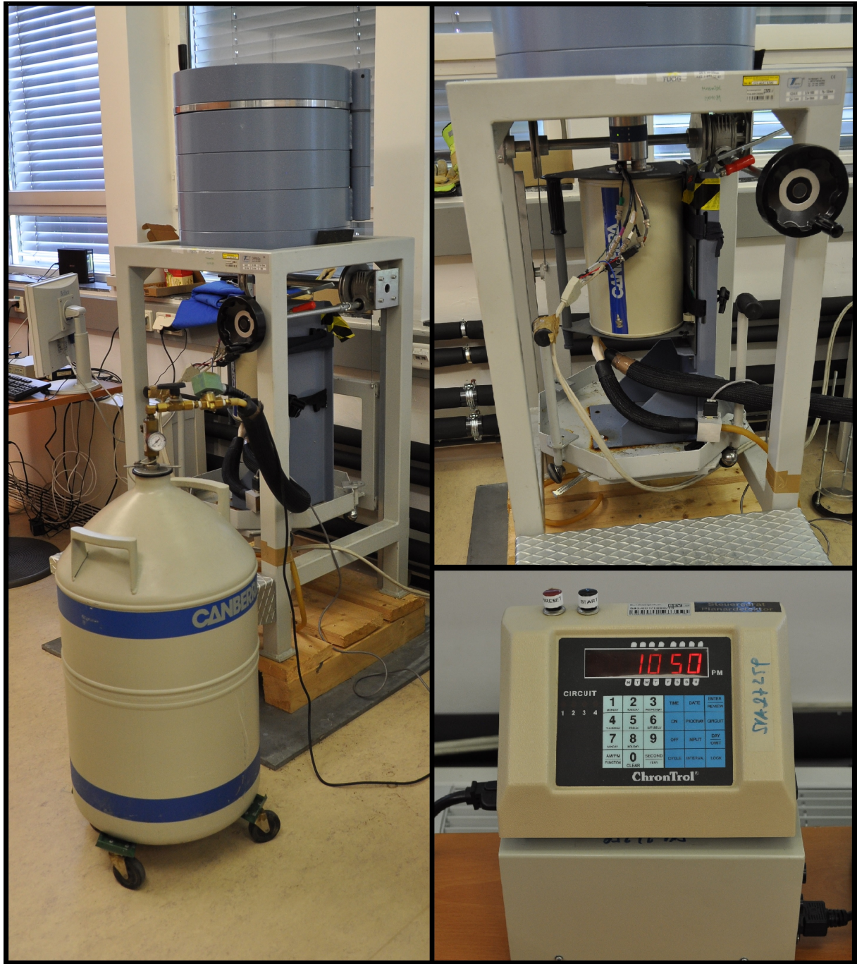
Figure 10.1.: Detector assembly of the Seibersdorf detector with liquid nitrogen container, dewar and timer for the automated cooling system
