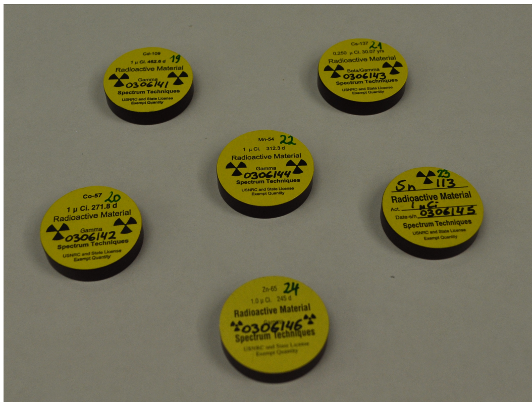
Figure 12.2.: Peak-to-total calibration source set
