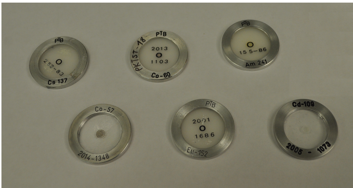
Figure 12.1.: Point sources used for energy calibration and establishing the detector parameters
