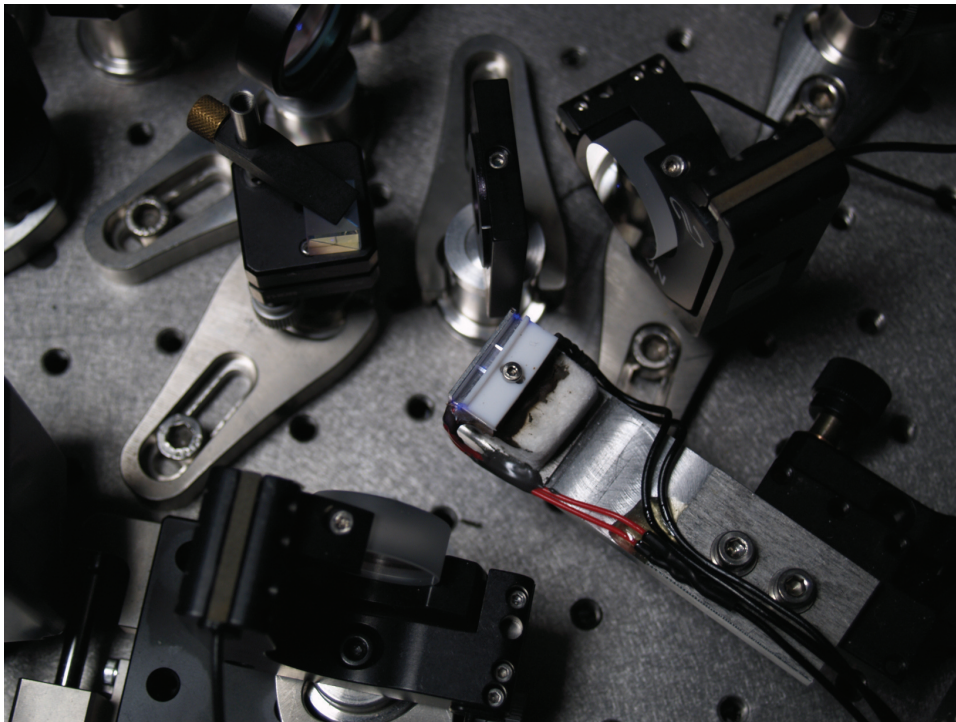
Figure 3.25: Close-up of the Sagnac loop in the Source. The crystal oven is longer than the crystal.
