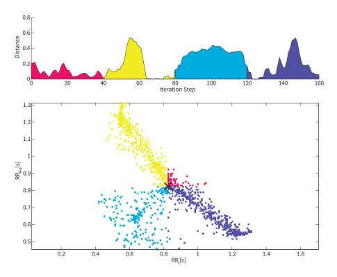
Figure 10: The distance function (top) and the corresponding Poincaré plot (bottom). The plot is scanned counter-clockwise and the mean value is marked with a black cross. The colors show the parts of the Poincaré plot with their equivalent area under the curve.
