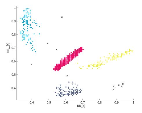
Figure 11: Clustered Poincaré plot of a subject with arrhythmia. The filter algorithm selected the cluster in red as the sinus beat cluster with the mean value marked as the gray cross. The other clusters and the noise (black crosses) are not considered for the calculation of the Poincaré plot indices, except for *NumberOfClusters* and *ClusterSizeRatio*.
