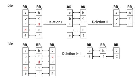
Figure 12: Deletion of the incorrect RR-interval "d" (Deletion I) and the corresponding counterparts "c" in RR<sub>1</sub> and "e" in RR<sub>1</sub> (Deletion II) for a 2D Poincaré plot. In the case of a 3D Poincaré plot for an erroneous interval "d", the preceding intervals "b" and "c" have to be deleted in RR<sub>1</sub>, "c" and "e" in RR<sub>2</sub> and "e" and "f" RR<sub>3</sub>.
