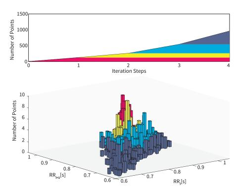
Figure 6: Approximated density function (top) with the corresponding 3D histogram (bottom) of a filtered non-pathologic Poincaré plot. Starting from the highest peak, the number of points in a certain neighborhood is summed up. The diameter of the this neighborhood is enlarged with each iteration, as shown color coded in the histogram and the density function.
