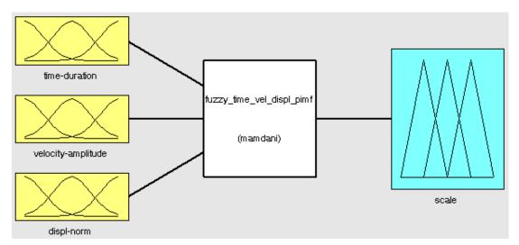
Figure 7.12: Feasible FIS in strength training with three input and one output parameters.
