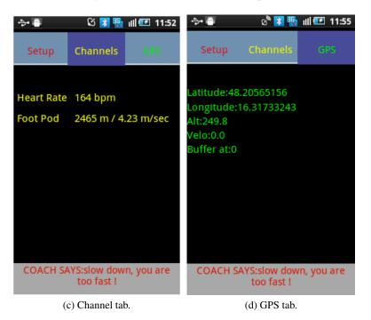
Figure 5.4: Implementation on an Android-based smartphone.
