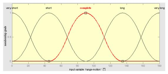
Figure 7.17: Exemplary fuzzy sets for the input variable representing the ROM.
