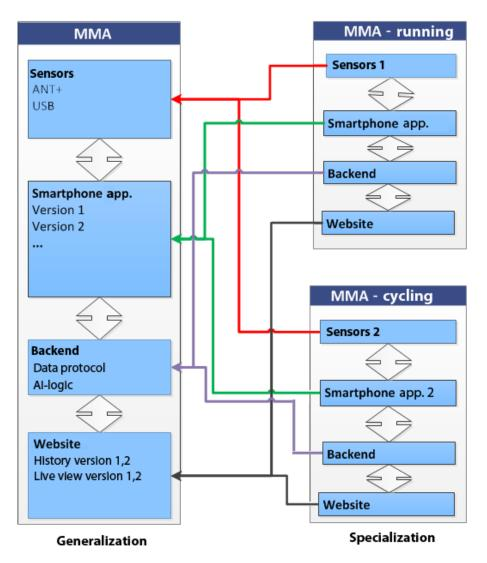
Figure 6.7: Generalization vs. specialization of the framework.
