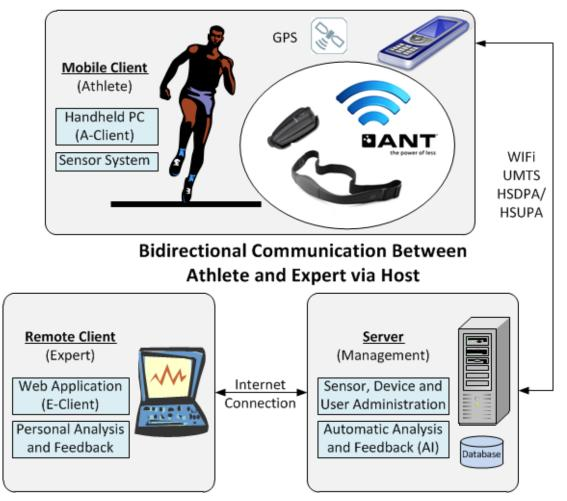
Figure 2.1: Overall concept of the system (bidirectional approach).
