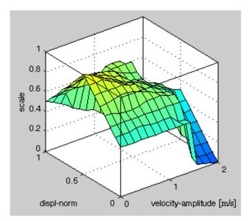
Figure 7.14: Relation between velocity amplitude, normalized displacement and respective scale values.
