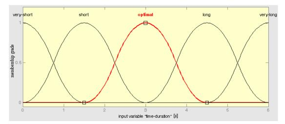
Figure 7.13: Exemplary fuzzy sets for the input variable mapping the time duration to a value between 0 (improper) and 1 (proper).
