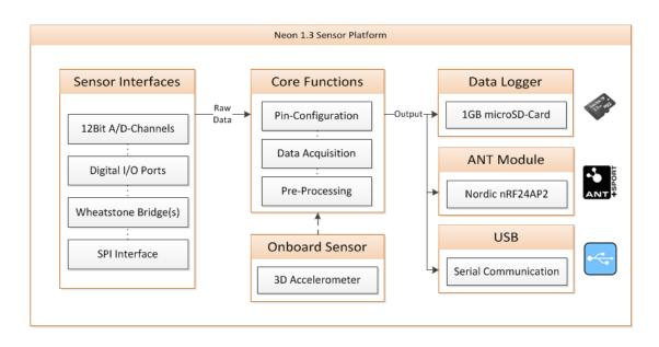
Figure 4.2: NEON sensor platform with integrated ANT chip.
