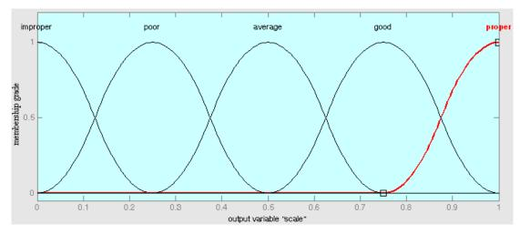
Figure 7.15: Exemplary fuzzy sets for output variable representing the overall rating (scale).
