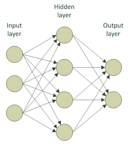
Figure 7.6: The typical design of an ANN with input, hidden and output layers, respectively consisting of three, four and two neurons.
