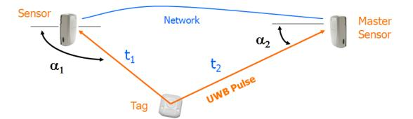
Figure 3.2: Position detection principle on the basis of gathered parameters like TDA and AOA (with permission from Ubisense, 2013).
