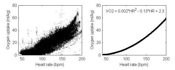
Figure 6.1: Illustration of the correlation between VO2 and heart rate (with permission from Saalasti, 2003).
