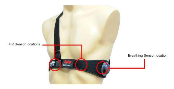
Figure 8.3: Appearance of the BioHarness chest strap with sensor locations (with permission from Zephyr, 2013b).
