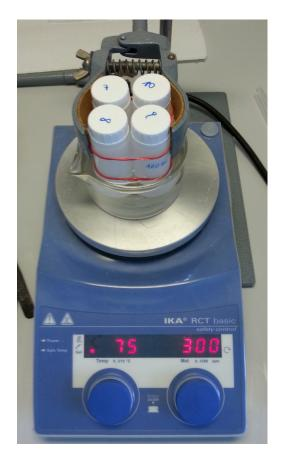
**Figure 3.7:** A metal clamp holds the four LSC bottles containing the  $HNO_3 + H_2O_2$  mixture and the TLD-600 dosimeters above a water bath. The bottles are dipped in far enough for the acidic mixture to be surrounded by water. The magnetic mixer is set to 75 °C and 300 rpm.
