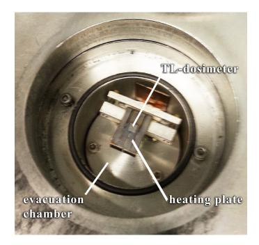
**Figure 3.5:** The evacuation chamber of the TL-DAT-III and the heat conducting plate within that chamber with a TL-dosimeter sitting on top of it.
