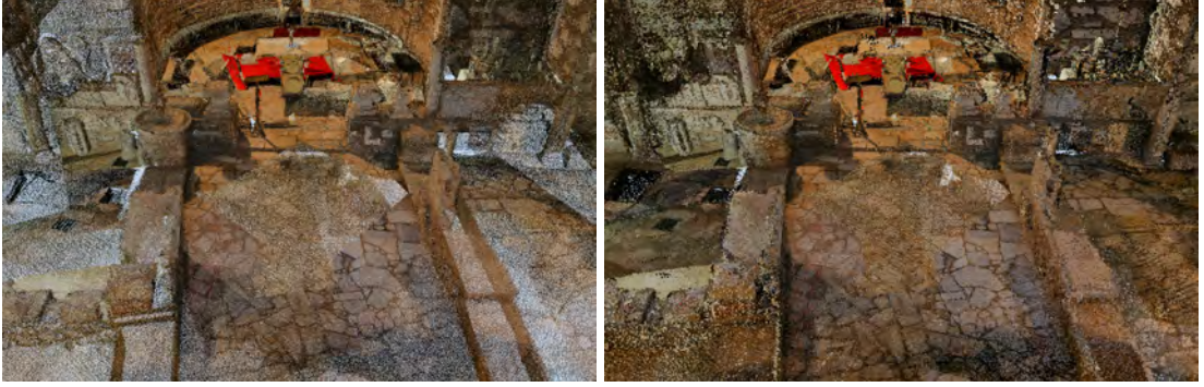
Figure 3.13: A view inside the basilica of the Domitilla catacomb model. On the left side, the point cloud is rendered with a fixed point size of one. The sparsely sampled areas are partly due to the different sampling densities, partly due to the LOD algorithm, which prefers to load nodes in the center of the screen. On the right side, the point cloud is rendered with the weighted point size. The level weight is calculated from the exact distribution of the points in the MNO.
