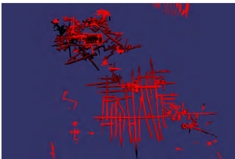
Figure 4.8: The second floor of the catacomb with elevation encoding. The height difference between pure red and black encoding is 3 meters.
