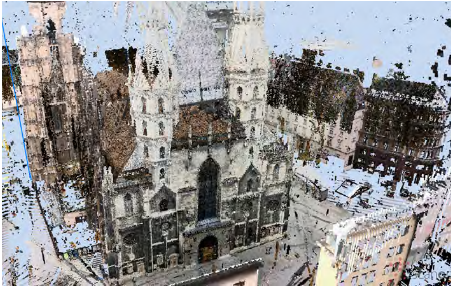
Figure 3.21: The Stephansdom model used for benchmarking the external sorting algorithms. It contains about 675 \cdot 10^6 points.
