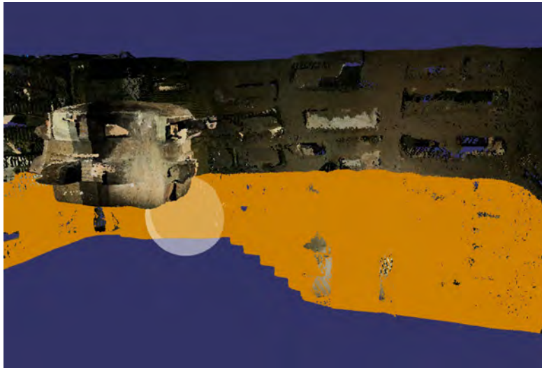
Figure 4.5: A close up view of a gallery in the region “Flavi Aureli”. Some areas are marked for deletion to gain a model of the initial building phase.
