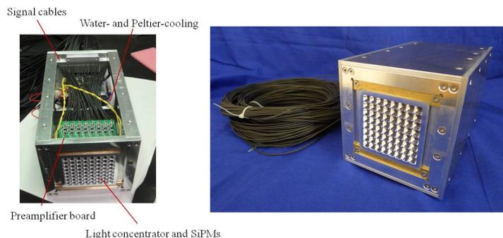
**Figure 1.** Pictures of the position sensitive SiPM array. The figure on the left shows a view inside the detector. The SiPMs are read out from the back by four preamplifier boards. The temperature is stabilized by water- and Peltier-cooling. The light guide matrix on top of the SiPMs enlarges the detection area of the module. On the right hand side the detector is closed.
