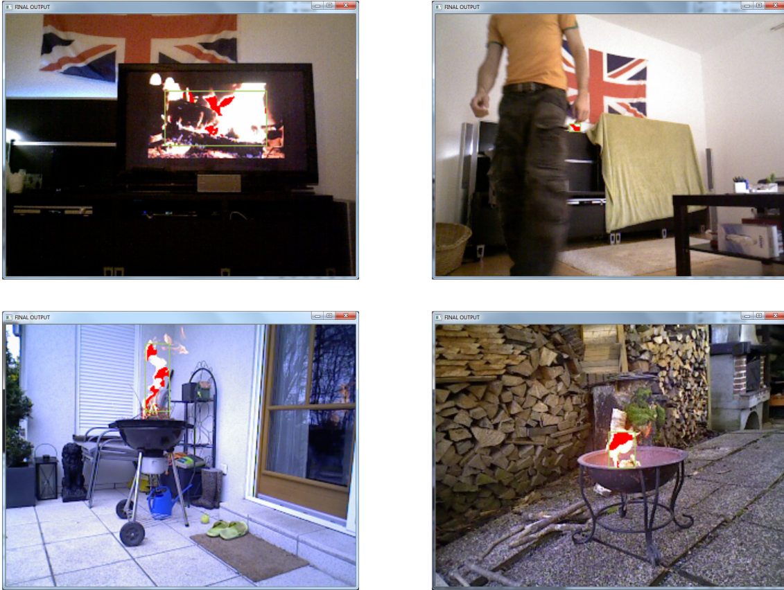
Figure 4.1: The top row shows frames from two videos that include motion and objects with a fire-like appearance. The image on the top-left shows the video of a fireplace replayed on a television. The image on the top-right shows someone dancing while wearing a fire-colored shirt. Both sample images on the bottom show real fire events. All videos have been recorded by the ASUS Xtion Pro.
