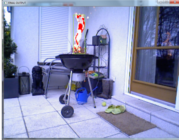
Figure 3.41: The implemented method for fire-detection, using the 2D RGB- and the 3D depth-sensor of the ASUS Xtion Pro. The analyzed regions are labeled as red (surrounded by a green rectangle).
