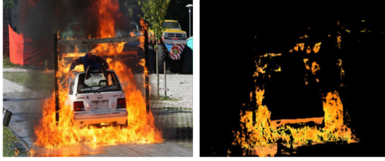
Figure 2.4: The image of a burning car before and after thresholding with RGB values [7].
