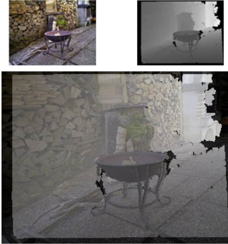
Figure 3.5: Two frames captured with the ASUS Xtion Pro. Image-registration was enabled while recording. Top-row, left: The captured RGB-frame. Top-row, right: The captured Depth-frame. Bottom-row: The superimposed image of RGB- and depth-camera. It can be seen that for example all edges are correctly arranged on top of each other.
