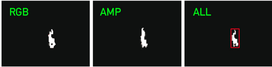
Figure 2.21: Left, the output (candidate region) of the fire detection algorithm using a RGB camera. The illustration in the middle visualizes the binary image, resulting from analyzing the amplitude image provided by the detection algorithm of sensor 2 . The right side shows the resulting frame, in this case the combination by a logical AND operator [29].
