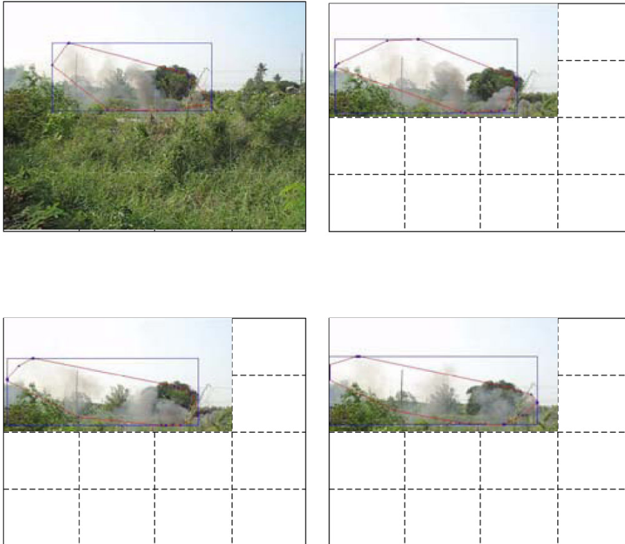
Figure 2.37: Clockwise, starting with the top-left picture: the results of the smoke-detection after one second, after 20 seconds, after 50 seconds and after 90 seconds [39].
