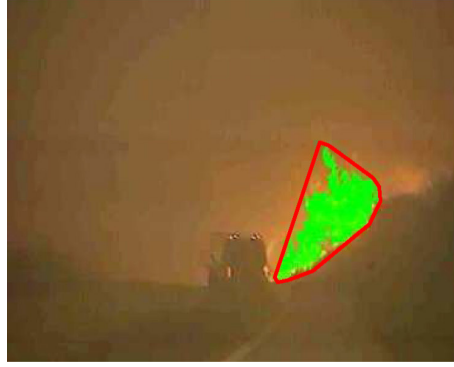
Figure 2.15: Due to the random shape of fire, a shape descriptor is calculated by using the ratio between the perimeter of the potential fire region and its smallest convex hull surrounding this area [5].
