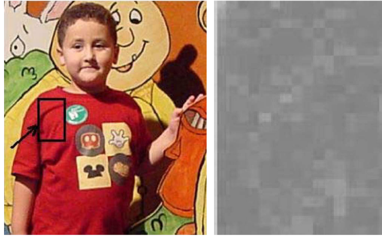
Figure 2.12: Left: a child with a fire colored shirt. Right: the wavelet image containing the accumulated, absolute values of the low-high, high-low and high-high wavelet transformations |LH_{(x,y)}| + |HL_{(x,y)}| + |HH_{(x,y)}| from pixels inside the rectangle [16].
