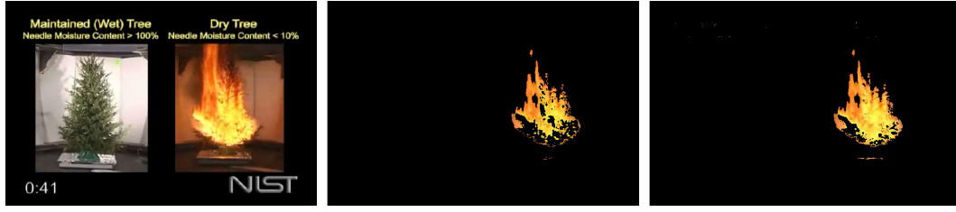
Figure 3.23: The analyzed frame_{(1380)} from video 5 on the left side. In the middle the image after restricting the color values as described in the section 'Color Range'. On the right side, the restriction of the blue color channel was relaxed from B < 80 to B < 100 .
