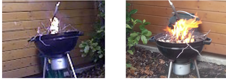
Figure 3.7: Two images from the same scene, left taken by the RGB camera of the ASUS Xtion Pro, right taken by the camera of a Samsung Galaxy S3. It can be observed that the ASUS Xtion Pro records fire as nearly white pixel
