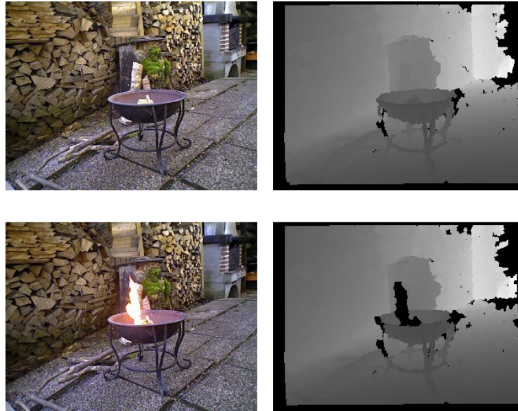
Figure 3.11: Two frames recorded by the ASUS Xtion Pro depth camera. Top row: frame_{824} recorded by the RGB and Depth camera, showing a scene without fire. Bottom row: frame_{11779} from the same scene. It can be seen that inside the fire-area the depth of the scene can not be calculated (illustrated by black pixel occurring in the depth-image).
