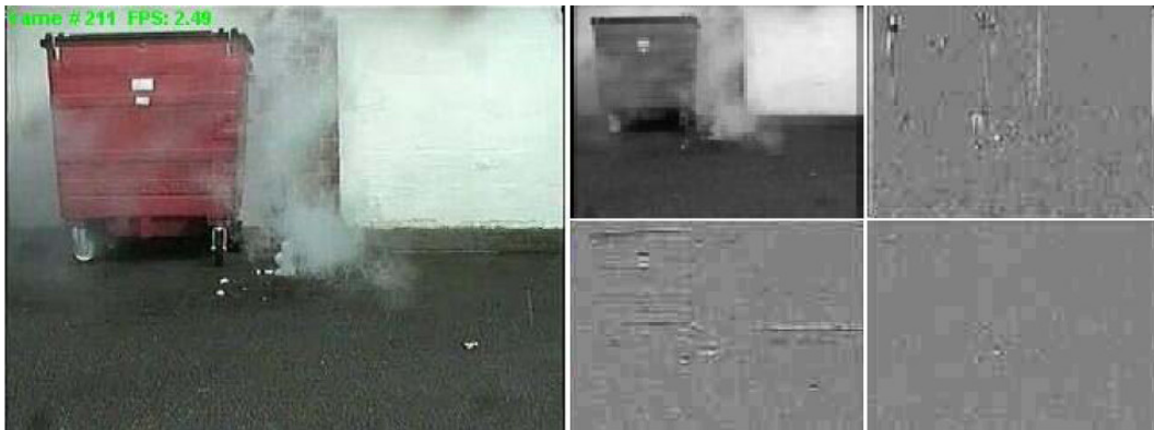
Figure 2.25: Left: the original frame. Right: the sub-images from the wavelet transformations, after a subsequent contrast enhancement. By comparing it to Figure 2.24, the decreasing variety of pixel-values in each sub-image can be recognized [13].
