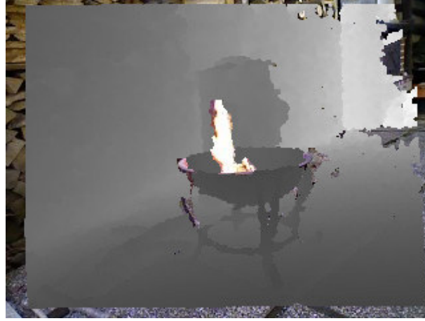
Figure 3.12: The superimposed image of RGB- and depth-camera from frame_{11779} , where black-pixels inside the frame of the depth-camera have been removed. It can be seen that the fire is located at the same area where the depth-camera is not able to calculate the depth of the scene.
