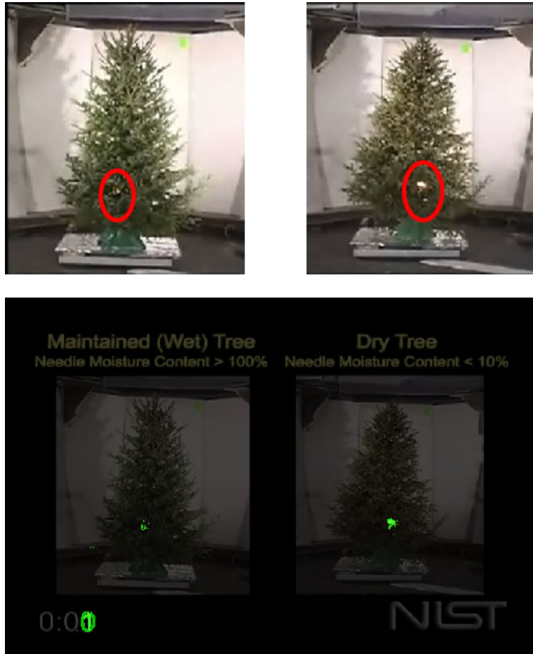
Figure 3.20: Frames from video 5 . The initial frame can be seen at frame_{(180)} at the top row (magnified), the bottom row shows an overlay of the same frame in original size, with pixel detected as moving highlighted.
