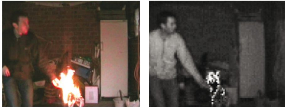
Figure 2.19: Fire that causes a high amount of disorder in the corresponding amplitude/intensity image [29].
