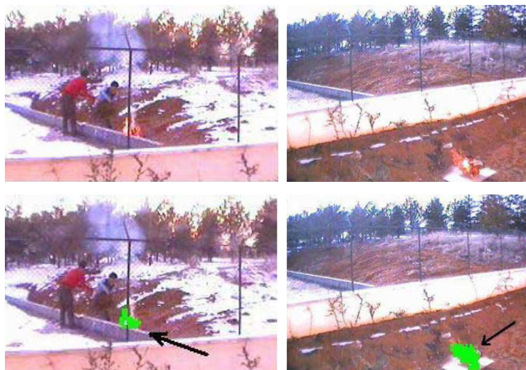
Figure 2.28: On the top: sample frames from two different movies. Bottom: the same frames processed with the proposed method, where all detected fire pixel have been highlighted in green [16].
