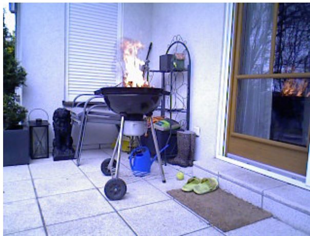
Figure 3.8: The image of a fire captured by an ASUS Xtion Pro with disabled Auto-White-Balance. It can be seen that the color-variation in the fire region is still very low.
