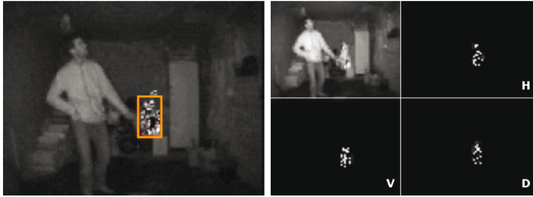
Figure 2.20: A captured amplitude image frame. The discrete wavelet transformation shows a high amount of disorder in the horizontal, vertical and diagonal analyzed sub-images, respectively [29].
