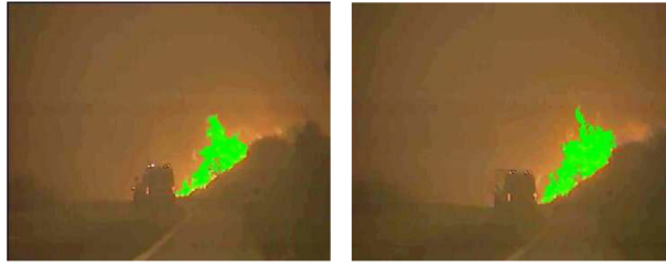
Figure 2.14: The difference of the area size between frame(i-1) and frame(i) , leading to a change from A_{i-1} = 1692 pixels to A_i = 2473 pixels [5].
