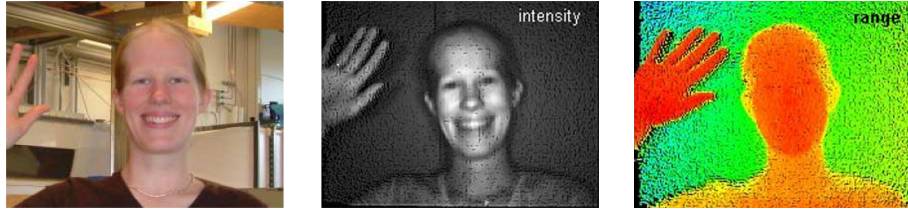
Figure 2.18: Left: a RGB frame, Middle: an amplitude image from the similar scene, showing the intensity of the received infrared light, Right: the calculated depth for the scene [32].
