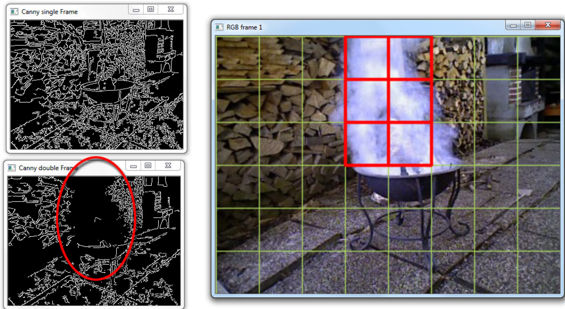
Figure 3.45: On the right side a RGB frame recorded by the ASUS Xtion Pro is shown. On the left side on top, the initially generated background image containing edges only is shown. The image below shows the edge-detection done by the same Canny-algorithm for the current frame. The region where smoke covers a significant amount of edges is marked in red.
