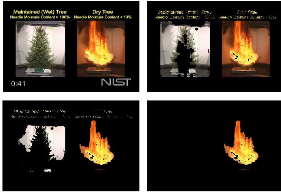
Figure 3.24: Top-row, left: the analyzed frame_{(1380)} from video 5 . Right: The same frame with restriction 1 applied, namely R > G > B . Bottom row, left: the same image using restriction 1 & 2, leading to (R > G > B) \wedge (R > \lambda_R) . Right: frame_{(1380)} again, with all three restrictions (R > G > B) \wedge (R > \lambda_R) \wedge (Saturation > \lambda_{Sat}) applied.
