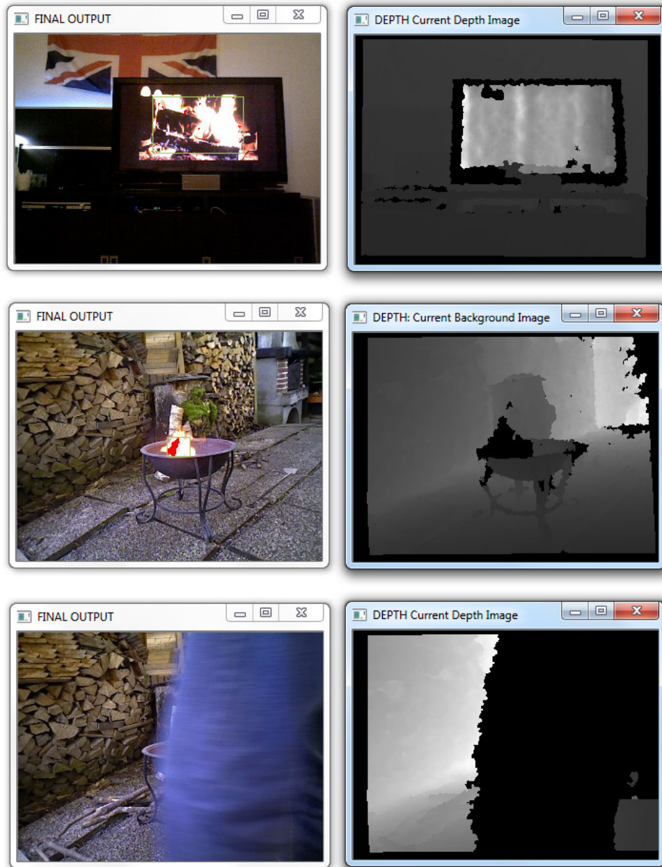
Figure 4.2: Left side: RGB-image. Right-side: Depth-image. The top row shows the impact of recorded fire to the color-sensor, while the depth-sensor is able to calculate a depth for the scene and therefore dismisses the fire-decision of the RGB-sensor. The second row shows the depth-image of the calculated background-image (not the current depth-frame as in row 1 and 3). Here, the missing region estimation can be clearly seen, because the recording of the fire was started after the fire was already burning. The last row shows the impact of a close-passing leg to the RGB-camera and the resulting problem estimating the depth in the depth frame.
