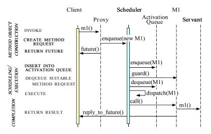
Figure 2.4: Sequence diagram of the different phases of an active invocation. [31]
