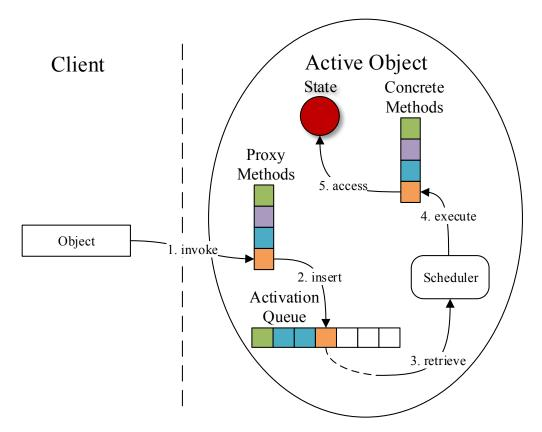
Figure 2.3: The control flow of a method call inside an active object.
