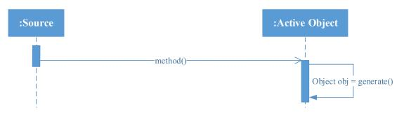
Figure 3.2: Sequence diagram of the purely asynchronous call mode.
