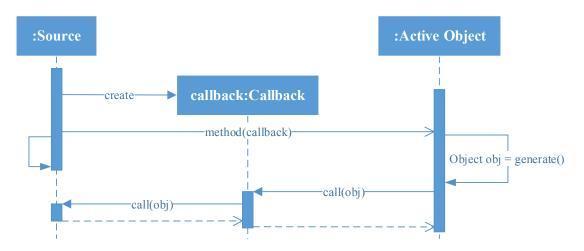
**Figure 3.3:** Sequence diagram of the asynchronous call mode based on a callback for result handling.
