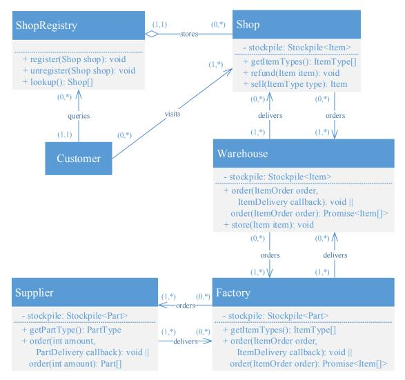
Figure A.1: The class diagram of the shop example.
