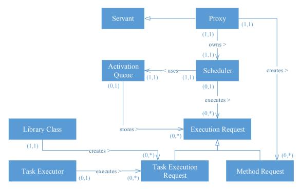
Figure 4.1: Class diagram depicting the relationships between the different core components.
