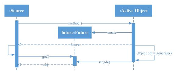
Figure 3.1: Sequence diagram of the asynchronous call mode using a future for result access.
