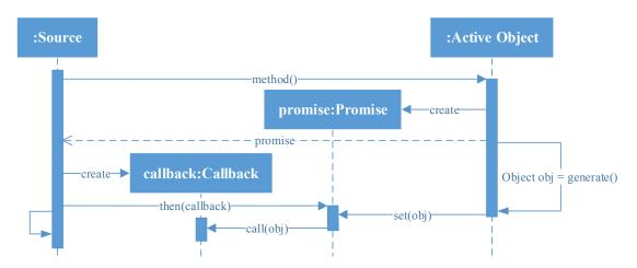
**Figure 3.4:** Sequence diagram of the asynchronous call mode based on a promise and a callback for result access.
