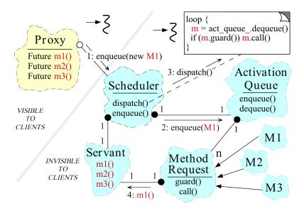
**Figure 2.2:** The original booch class diagram that shows the key components of the active object pattern. [31]
