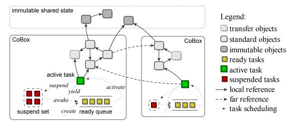
Figure 2.5: The various components of the JCobox model. [45]
