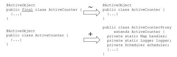
Figure 5.4: A number of code transformations necessary for the creation of the proxy class.
