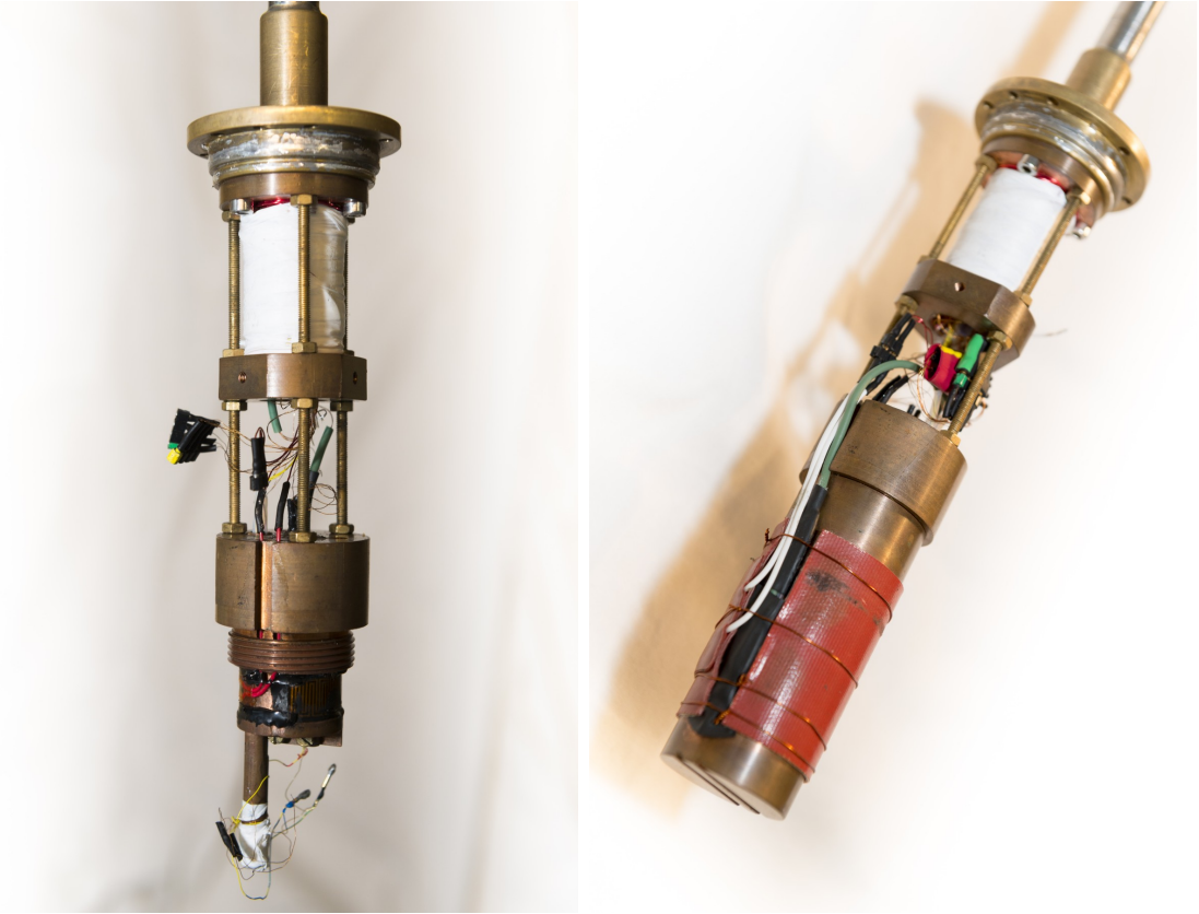
(a) ‘Open’ sample holder without sample (b) Finished assembly, without vacuum cup
