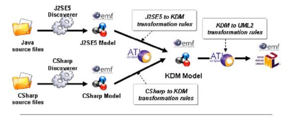
Figure 5.4: MoDisco standard transformation chain [38].
