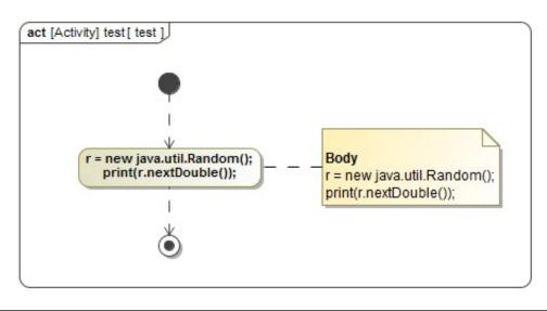
Figure 9.1: NoMagic MagicDraw Cameo Simulation Toolkit external library call specification.
