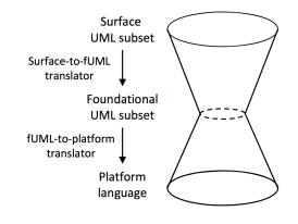
Figure 3.1: Translation to and from the foundational UML subset [31].
