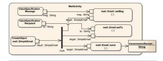
**Figure 4.3:** Modeling the UML activity model referencing the ApacheMail external library (step 3).
