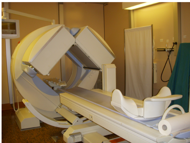
Figure 2.2: Picture of a gamma camera present at the MedUni Vienna. The two gamma camera blocks are rotated around the patient for 3D imaging [Figure: Courtesy of A. Hirtl].
