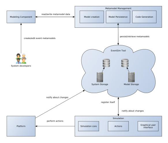
Figure 4.1: Architecture of the EventSim framework
