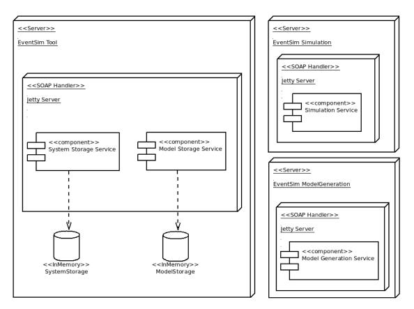
Figure 5.1: Deployment diagram of the EventSim framework
