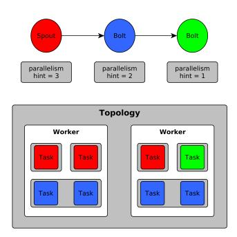
Figure 2.5: Example of a Storm topology
