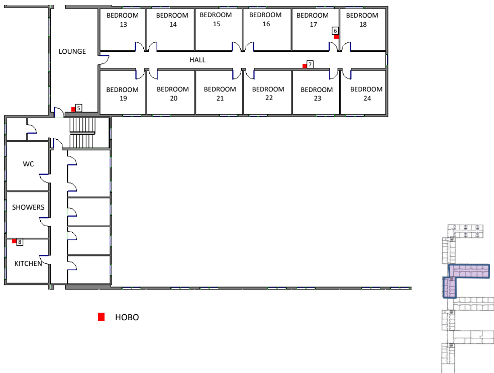
Figure 4 Data loggers (HOBO) on the First Floor
