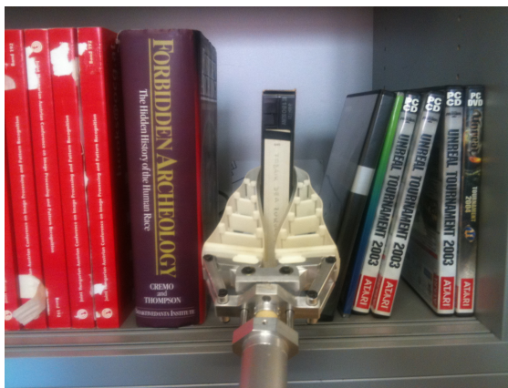
Figure 6.1: Motivation of pre-grasp gripper opening width: The picture shows a scenario where an initially fully opened gripper could not succeed, because gripper-object collisions would occur while approaching the final grasp position.
