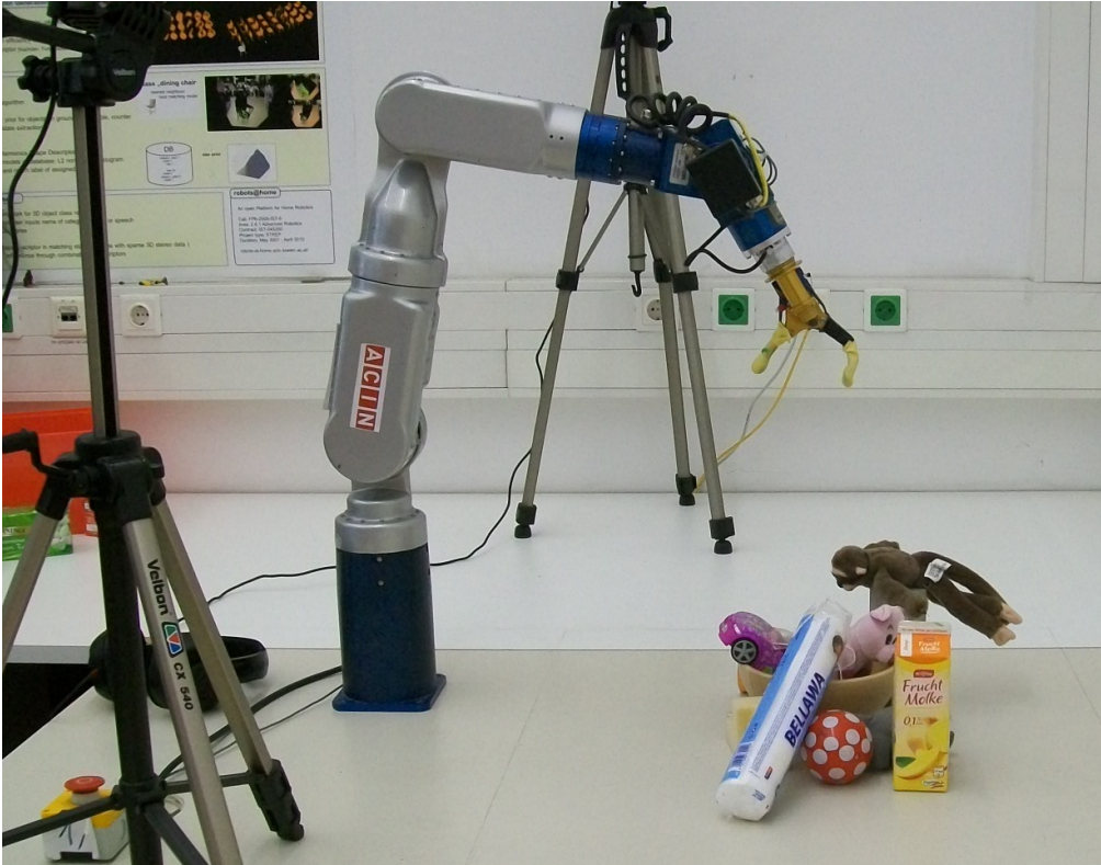
Figure 8.2: The 7-DOF Schunk arm and the tripods for the two cameras used for the clearing the table experiments.
