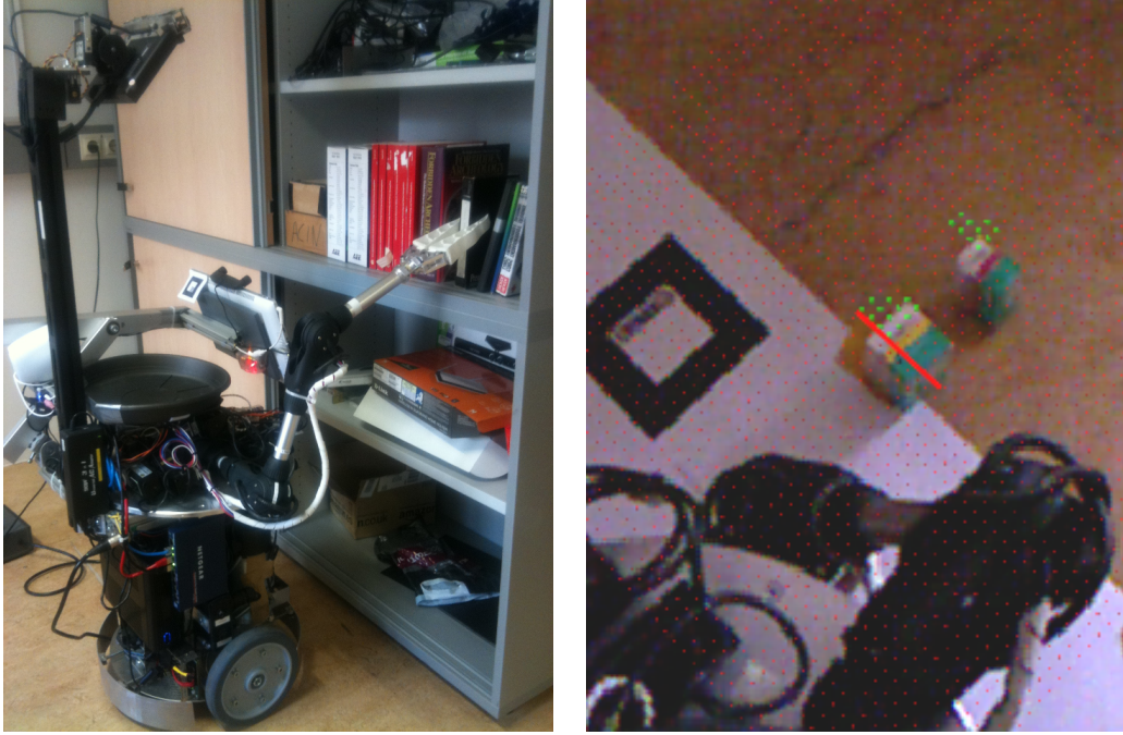
(a) Hobbit is grasping a tape in a scenario (b) Grasp grid results for one orientation and where a fully opened gripper would not succeed.
