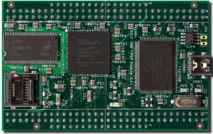
Fig.11: Picture of ZTEX USB-FPGA-Module 1.11c [8]
