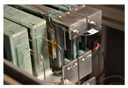
Figure 8.21.: The full-scale modules are cooled using the prototype open  $CO_2$  cooling system.
