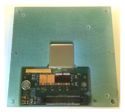
Figure 7.11.: A beam test module holding a baby sensor is opened to reveal the sensor's n-side and the front-end readout electronics (i.e. the hybrid board housing the APV25 chips). The strips of the sensor are connected to the APV25 chips via a glass pitch adapter.
