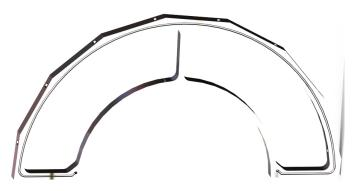
Figure 2.5.: Half of layer 6 backward end-ring, exposing the cooling channel. The end-rings arrange the ladders cylindrically around the beam pipe.
