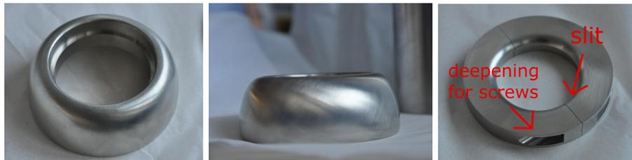
**Figure 3.13:** Photographs of the re-designed top cover of the electrode e17: left and middle: outer ring, right: two half rings which are pushed inside the outer ring.
