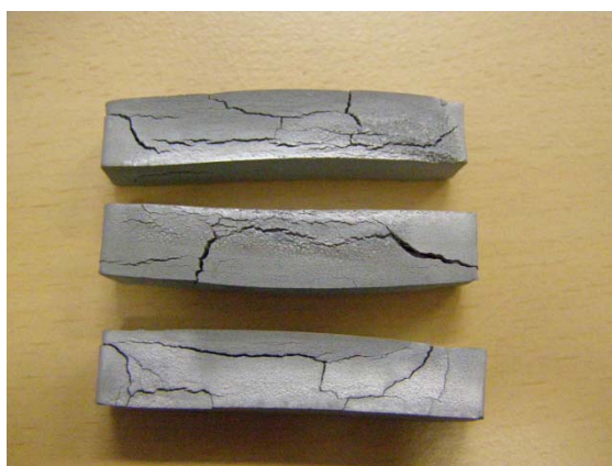
fig. 3.34.: Macroscopic view of sintered specimens. During sintering cracks occurred which destroyed the samples
