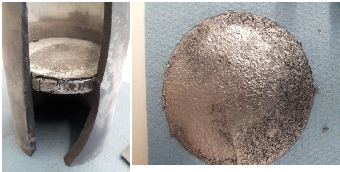
fig. 3.68.: Left: hot pressed sandwich-structured sample embedded in graphite die; right: disc-shaped structured sample after HP without carbon die (punch surface)
