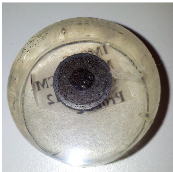
fig. 3.81.: Embedded sample; 3 different layers can be observed
