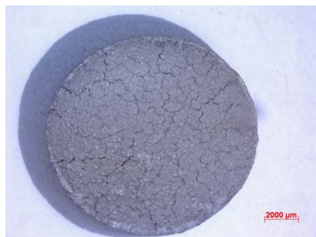
fig. 3.40.: Specimen Mo + 5 wt % EBS after sintering covered with cracks
