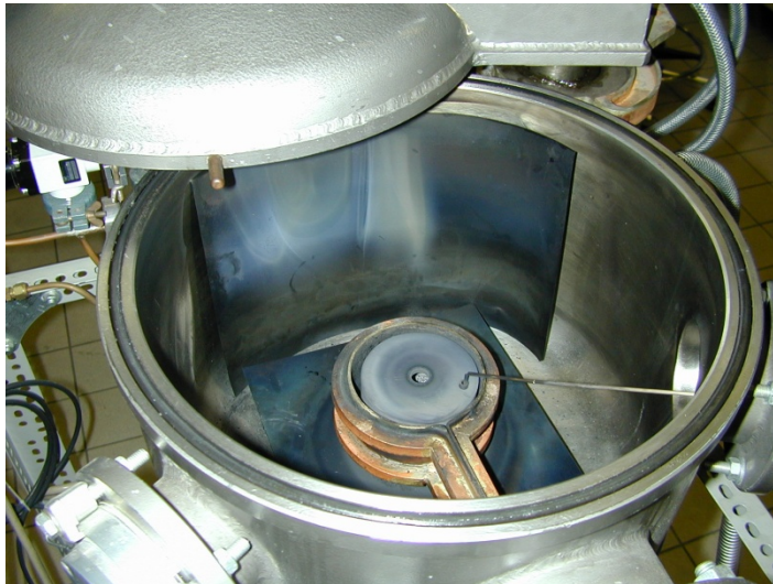
fig. 2.11.: inside of the MF - recipient - induction furnace
