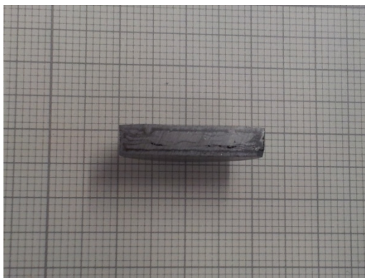
fig. 3.42.: camera picture of the cross section of Mo specimen with 5 wt% space holder sintered
