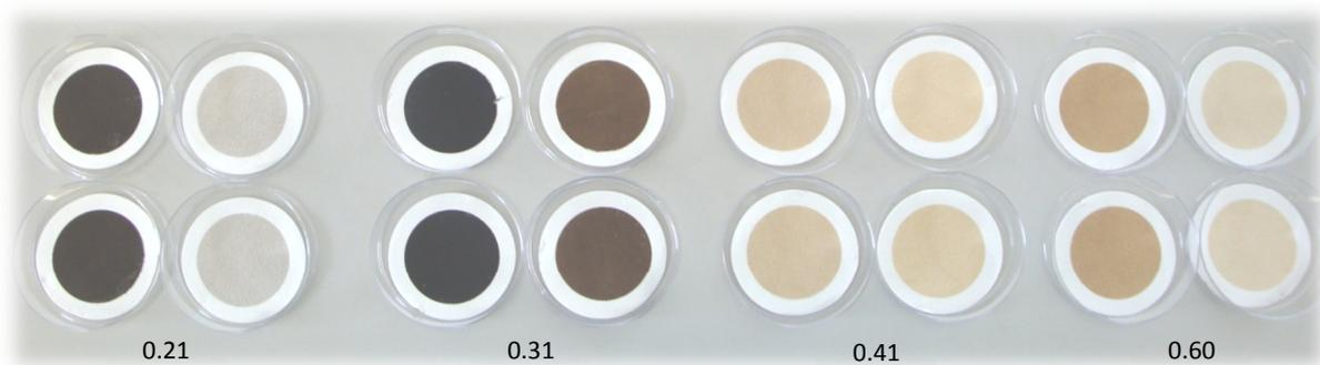
*Figure 14: Four sets of filters under different operating conditions. The left pair in the set was sampled when no mixing gas ( $N_2$ ) was present, as opposed to the right pair. The first group of four filters had a C/O ratio of 0.21, the second 0.31, the third 0.41 and the last group 0.60 (left to right).*
