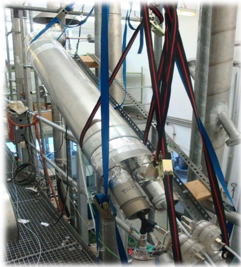
Figure 31: Dilution/cooling pipe with two-particle separators ( $PM_{10}$  and  $PM_{2.5}$ ) and filter holders.
