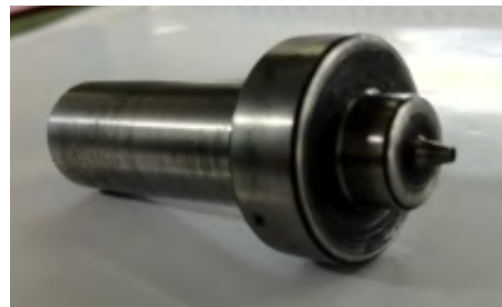
Appendix A-2: Blueprint and picture of tool with a shoulder diameter of 12 mm
