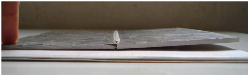
Appendix A-30: Distortion of the LHW specimen due to thermal stresses
