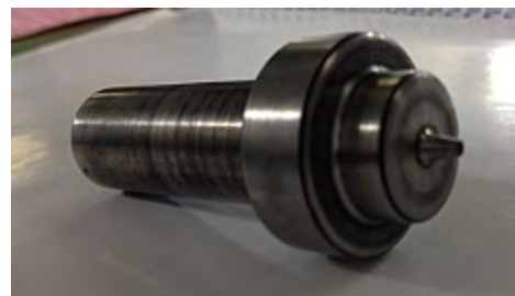
Appendix A-3: Blueprint and picture of tool with a shoulder diameter of 16 mm
