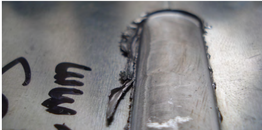
Appendix A-12: Flash alongside the weld of specimen 5
