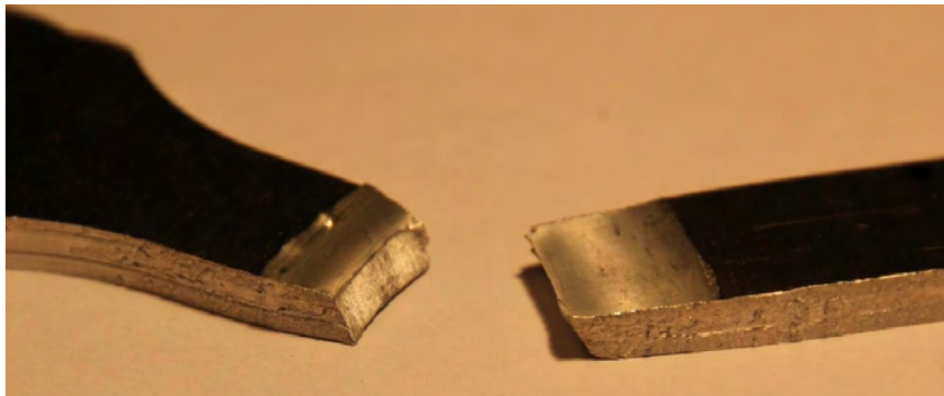
Appendix A-16: Tensile specimen of the FSW weld 7 after fracture
