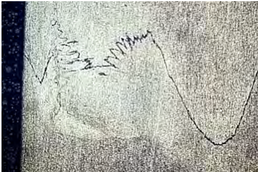
Appendix A-26: Diagonal macroetch of specimen 4, revealing a root flaw on the left the oxide layer at the edges of the joint result in the wavelike inter-phase
