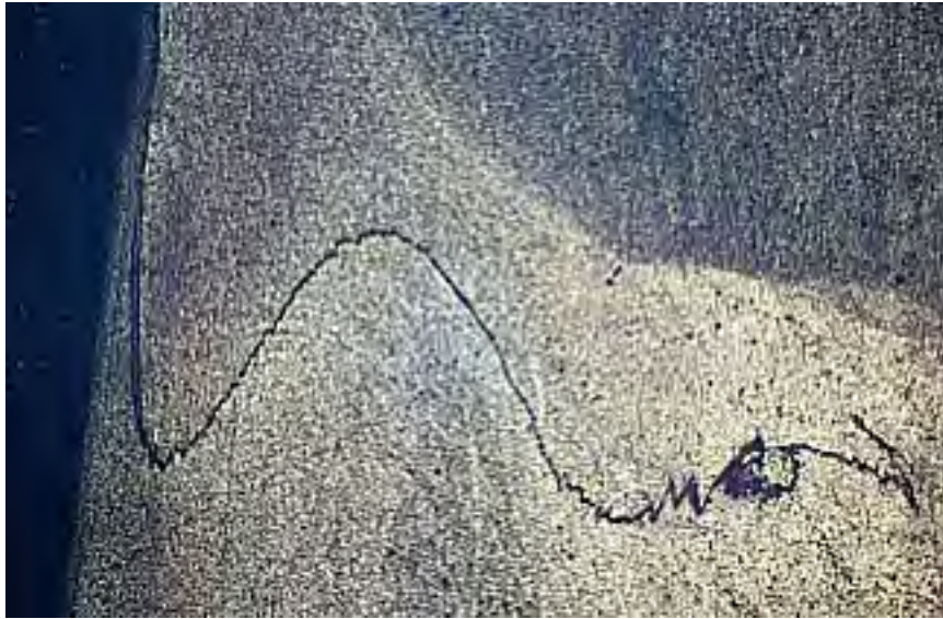
Appendix A-25: Transversal macro-etch of specimen 4: the brighter region represents the dynamically recrystallized zone DXZ; the oxide layer at the edges of the joint result in the wavelike inter-phase
