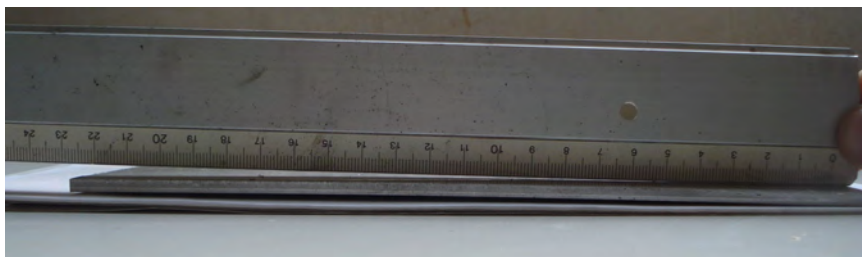
Appendix A-31: Distortion of the LHW specimen due to thermal stresses
