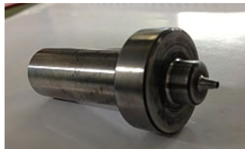
Appendix A-1: Blueprint and picture of tool with a shoulder diameter of 10 mm
