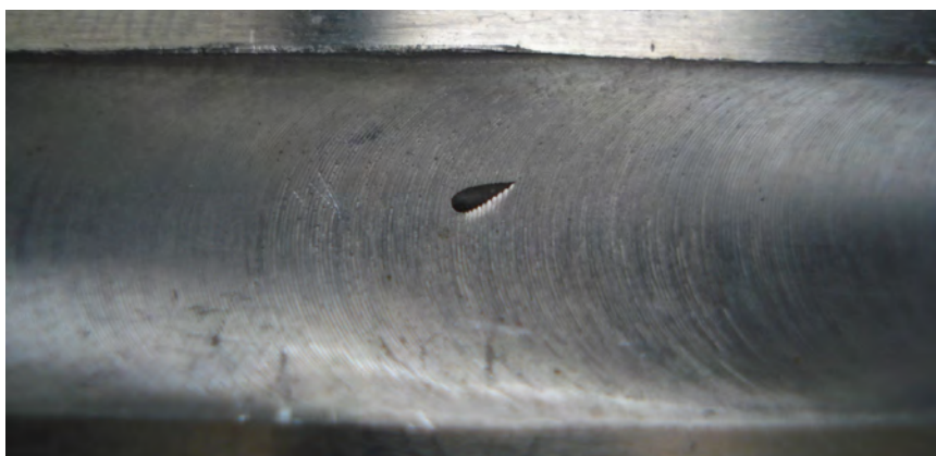
Appendix A-14: A cavity on the face side of FSW specimen 7
