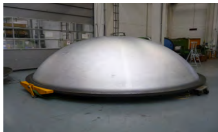
Figure 1-1: The dome of a space shuttle fuel tank produced using FSW technology [1]
