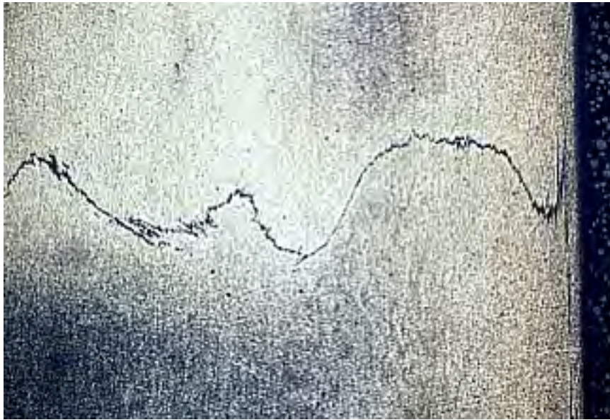
Appendix A-23: Transversal macro-etch of specimen 3 : the oxide layer at the edges of the joint result in the wavelike inter-phase
