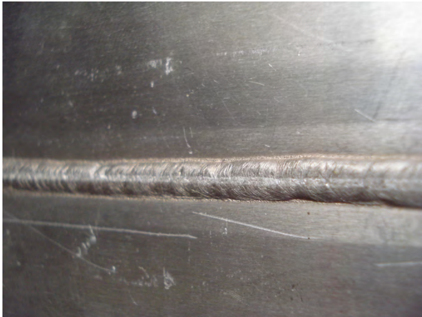
Appendix A-29: Close-up of root of LHW specimen; HAZ is represented by the bright region along the weld root
