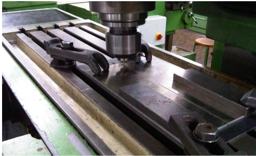
Appendix A-6: Securing of the workpieces with clamps before Welding
