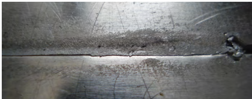
Appendix A-11: Root side of FSW specimen 2: material discontinuity at the start of weld
