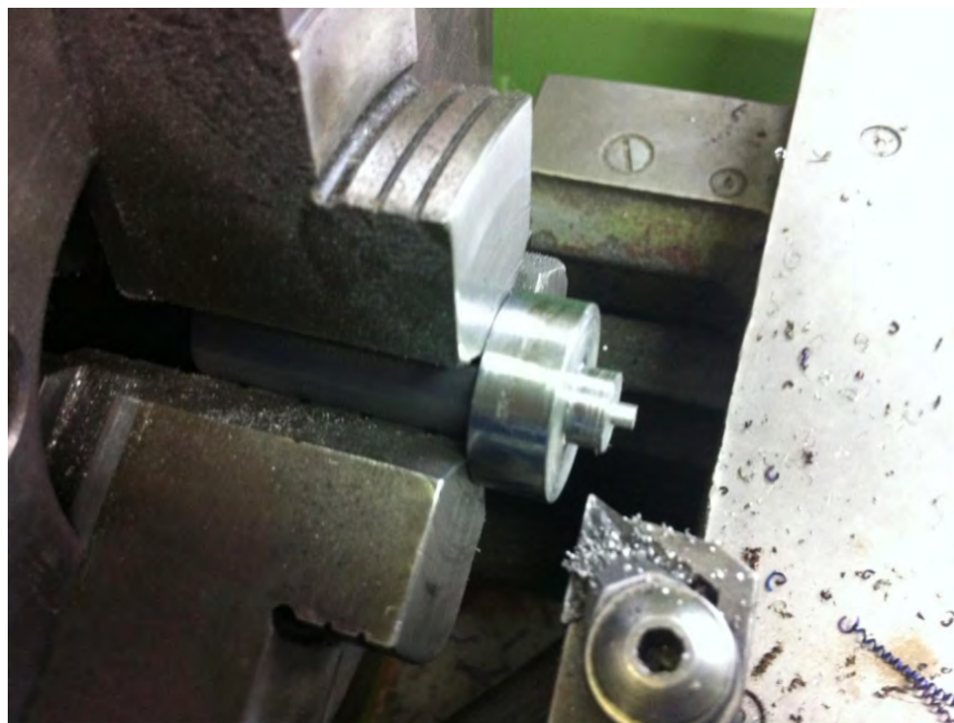
Appendix A-5: Machining of the FSW tools
