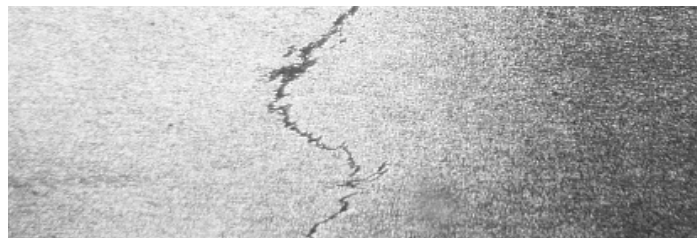
Figure 4-16: Joint line remnant in an FSW weld
