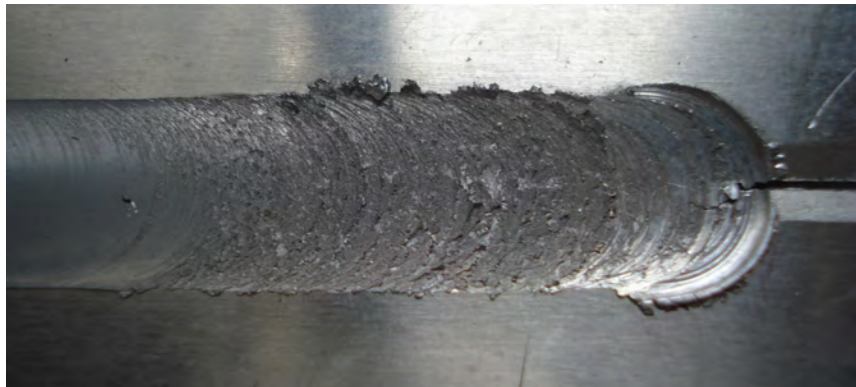
Appendix A-10: Face side of FSW specimen 2: irregular welding pattern and a small crack at the start of weld
