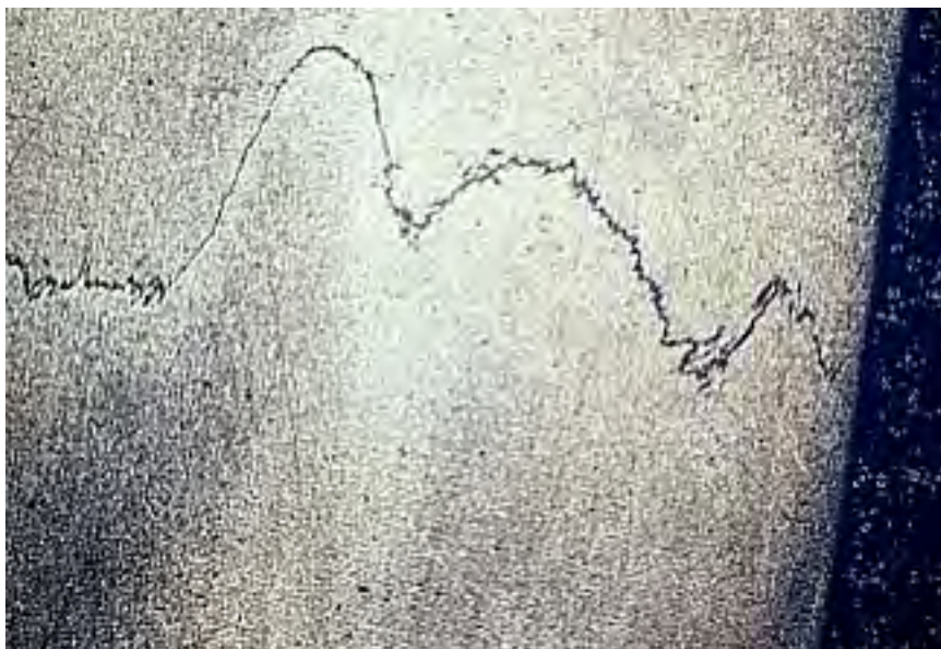
Appendix A-24: Diagonal macroetch of specimen 3 revealing a root flaw on the right the oxide layer at the edges of the joint result in the wavelike inter-phase
